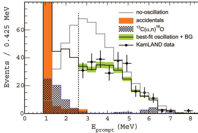
**Figure 2.** Observed energy spectrum of the reactor anti-electron-neutrino interactions observed in KamLAND is compared with the expected spectrum with and without neutrino oscillations. The estimated background events are also shown. The dashed line shows the threshold of the analysis (2.6 MeV).
