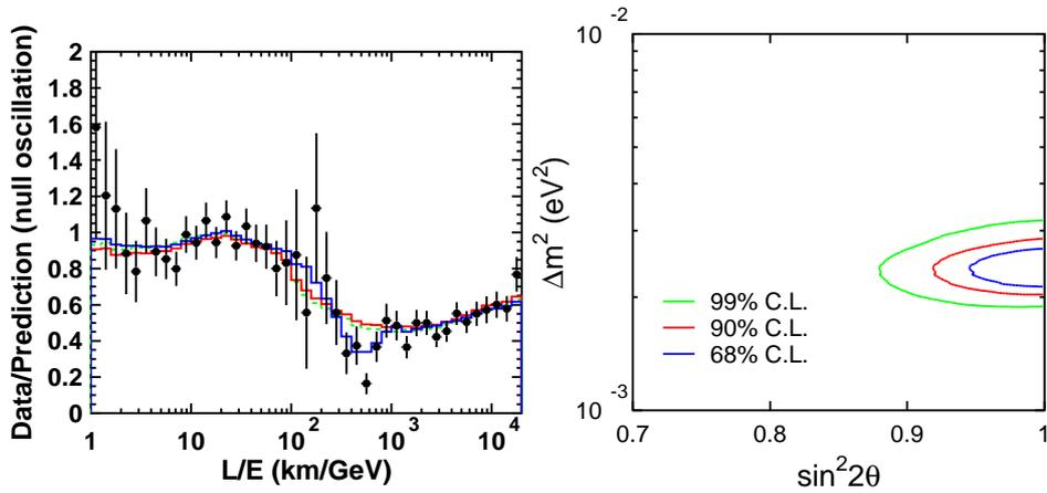
**Figure 6.** Left:  $L/E$  distributions observed in Super-K-I and Super-K-II (1489 and 627 days, preliminary). Right: Allowed oscillation parameter regions from the  $L/E$  analysis of the Super-K-I and Super-K-II data (preliminary).
