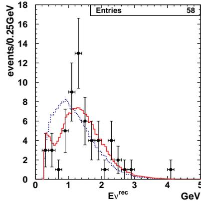
**Figure 8.** Reconstructed neutrino energy spectrum in K2K using 58 single-ring  $\mu$ -like events. The dotted and solid histograms show the predicted spectrum for no oscillation and  $\nu_\mu \rightarrow \nu_\tau$  oscillations. The histograms are normalized by the number of observed events.
