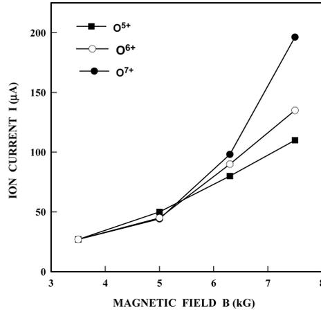
**Figure 3.** Comparison of the normalized curves for the oxygen ions showing steepness of the curves.
