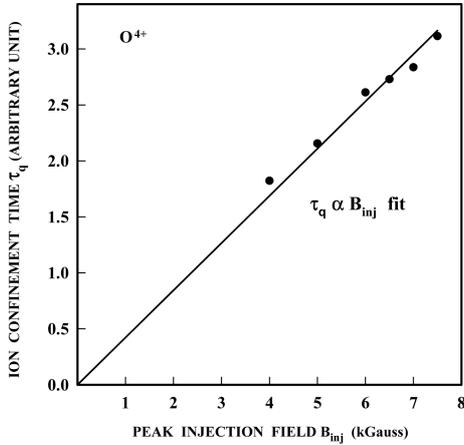
**Figure 6.** Variation of the calculated average confinement time of  $O^{4+}$  ions on the peak injection field. The line is a fit passing through the origin.
