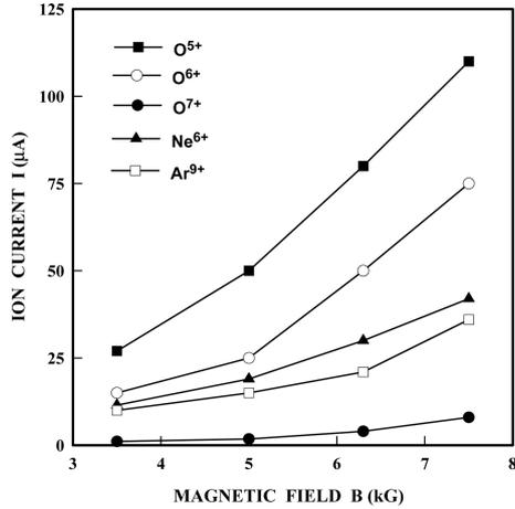
**Figure 2.** Extracted ion current from 6.4 GHz VEC-ECR source for different charge states of various species.
