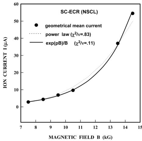
**Figure 9.** Comparison between various fits for SC-ECR of NSCL. The solid circles are the geometrical means of the current values shown in figure 8.
