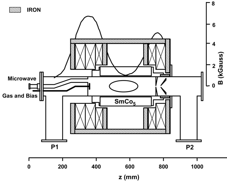
**Figure 1.** The 6.4 GHz ECR ion source at VECC, Kolkata.
