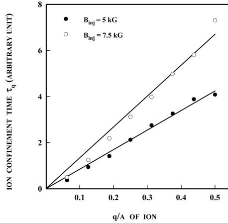
**Figure 7.** Dependence of the average confinement time of ions on charge-to-mass ratio.
