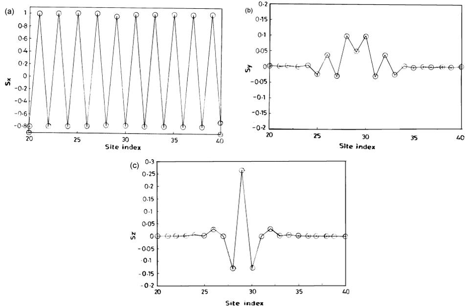
**Figure 7.** (a) Plot of  $S_x$  vs.  $n$  in an easy-plane ferrimagnetic system. The parameters are:  $J_x = J_y = J_z = -0.1, D = -1.0, S = 0.8$ . (b) Plot of  $S_y$  vs.  $n$  for the same choice of parameters. (c) Plot of  $S_z$  vs.  $n$  for the same choice of parameters.
