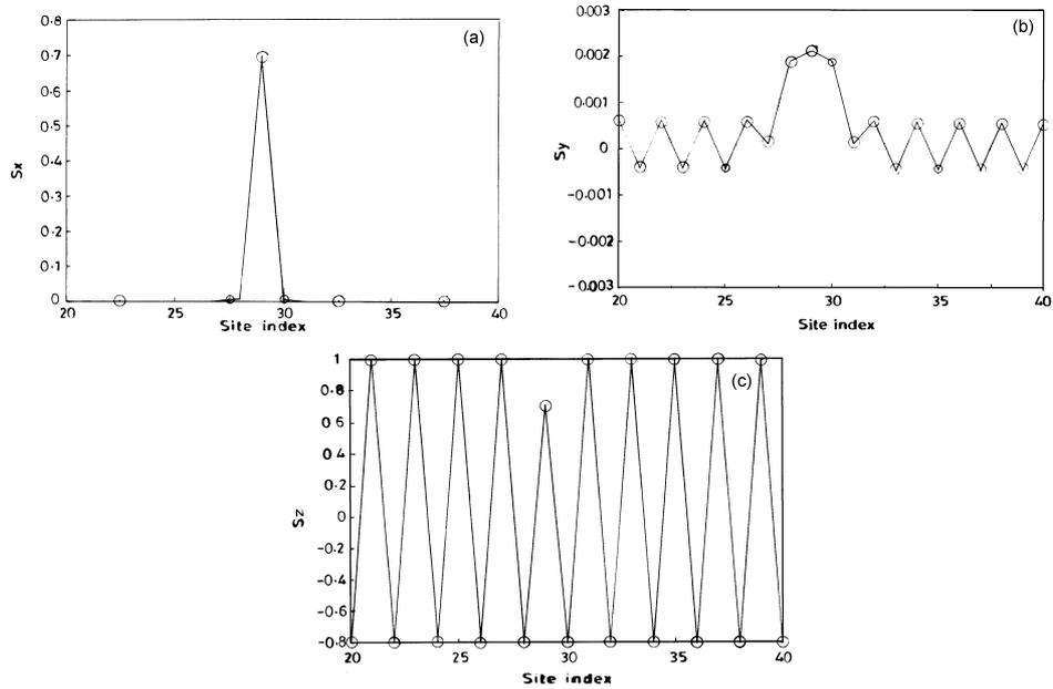
**Figure 6.** (a) Plot of  $S_x$  vs. site index  $n$  for the parameters:  $J_x = J_y = -0.1, J_z = -1.0, D = 1.0, S = 0.8$ . (b) Plot of  $S_y$  vs.  $n$  for the same choice of parameters. (c) Plot of  $S_z$  vs.  $n$  for the same choice of parameters.
