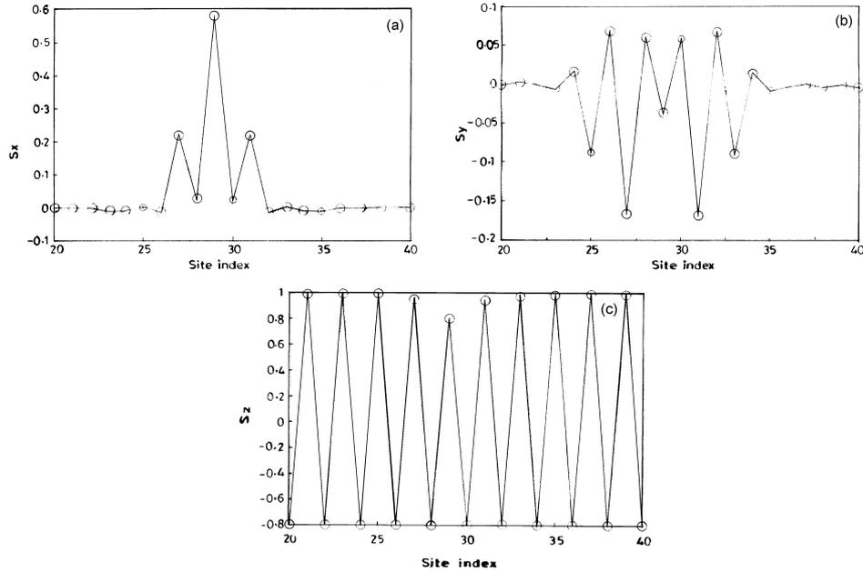
**Figure 5.** (a) Plot of  $S_x$  vs. site index  $n$  for coloured breathers in an easy-axis ferrimagnetic system obtained by solving the time evolution equation by Runge–Kutta method. The parameters are:  $J_x = J_y = J_z = -1.0$ ,  $D = 1.0$ ,  $S = 0.8$ . (b) Plot of  $S_y$  vs.  $n$  for the same choice of parameters. (c) Plot of  $S_z$  vs.  $n$  for the same choice of parameters.
