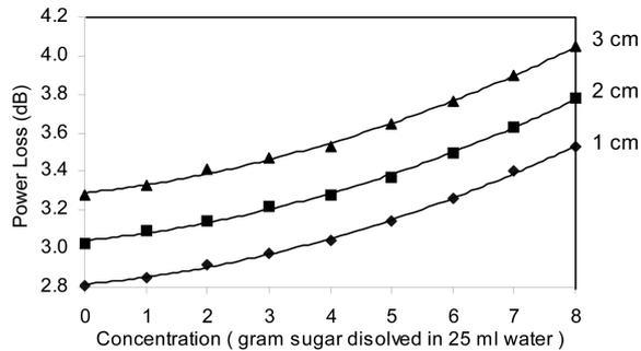
**Figure 3.** Graph showing concentration vs. power loss at 850 nm for 1, 2, 3 cm core exposed in sugar solution in plastic fiber.
