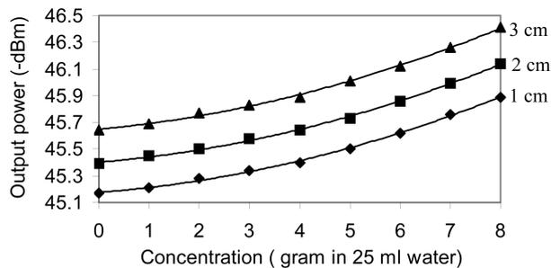
**Figure 2.** Graph showing concentration vs. output power at 850 nm for 1, 2, 3 cm core exposed in sugar solution in plastic fiber.
