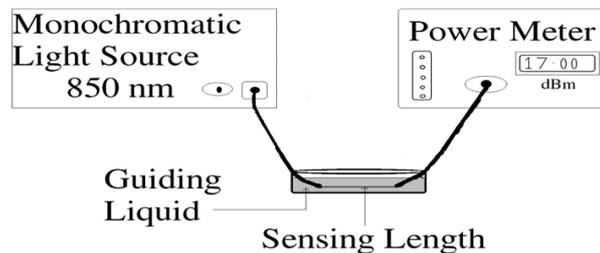
Figure 1. Experimental arrangement of the fiber optic sensor.
