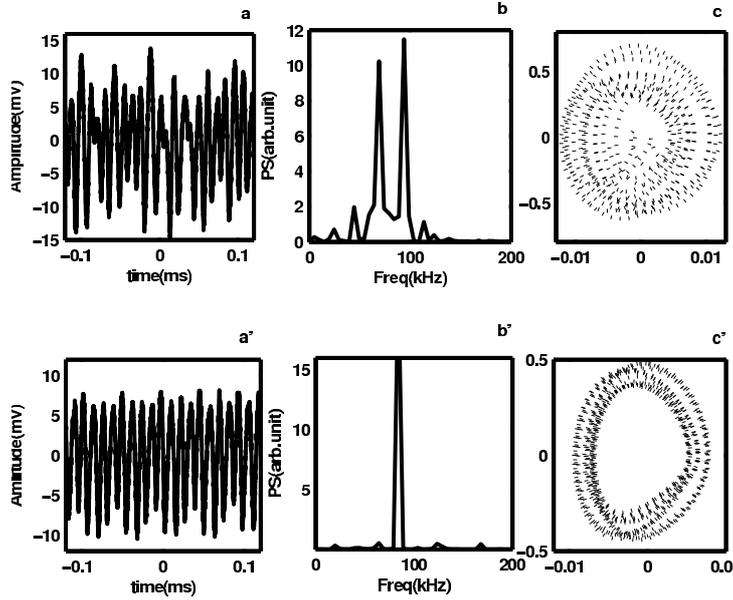
**Figure 3.** (a,a') Raw data, (b,b') power spectrum and (c,c') phase space plots at 284 and 286 V respectively. Through period subtraction the system attains five period at a discharge voltage of 286 V from the seven period state at a voltage of 284 V.
