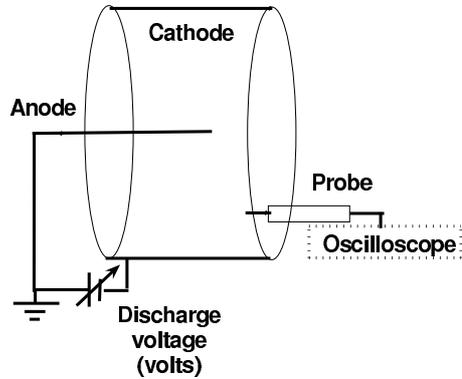
**Figure 1.** Schematic diagram of experimental set-up of cylindrical DC discharge plasma system with Langmuir probe fitted with digital oscilloscope. A DC voltage has been applied to the cathode (outer cylindrical surface) with respect to the grounded coaxial cylindrical rod and plasma is formed inside it.
