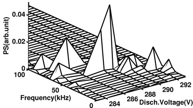
**Figure 7.** Changes of power and frequencies with discharge voltages.  $X$ -Axis represents discharge potential,  $y$ -axis represents frequencies, and  $z$ -axis represents power spectrum (PS) of the signals at different discharge voltages. With increase in the discharge voltage low modes appear.
