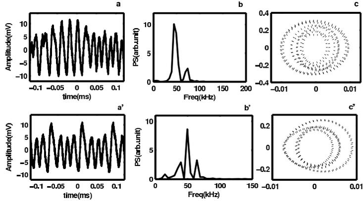
**Figure 5.** Further increasing the voltage the system goes through two successive bifurcations. The sequences (a) → (b) → (c) and (a′) → (b′) → (c′) show that mode appears at 290 and 291 V respectively due to bifurcation.
