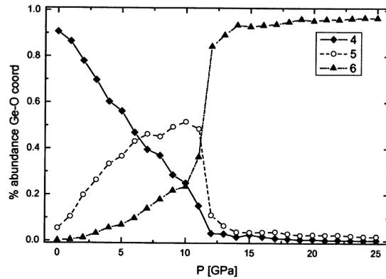
**Figure 12.** Variation of fractional abundance of Ge–O coordination with pressure for the phase which was liquid at 1650 K.
