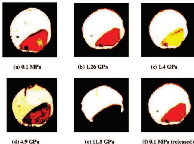
**Figure 6.** Microphotographs of HgI<sub>2</sub> single crystal in the gasketed diamond anvil cell taken at different pressures (a–f). The circular spot in (a) indicates the typical size of the monochromatic beam focused onto the sample. At 1.3 GPa initially red crystal turns yellow.
