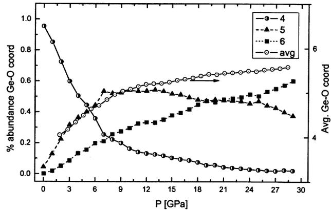
**Figure 9.** Variation of fractional abundance Ge–O coordination with pressure for vitreous GeO<sub>2</sub> at 300 K.
