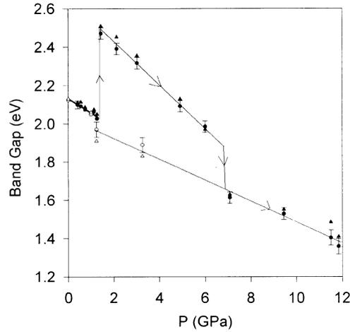
**Figure 7.** Pressure dependence of the band gap in HgI<sub>2</sub>. Band gap increases abruptly at 1.4 GPa (direct–direct transition) followed by another (direct–indirect transition) at ~7.0 GPa. Upon release of pressure, the observed changes in the gap do not retrace the changes observed on pressure increase.
