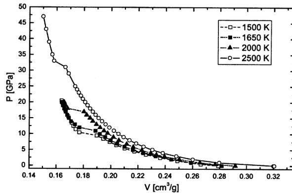
**Figure 10.** Variation of the volume of molten GeO<sub>2</sub> on increase of pressure at 1500, 1650, 2000 and 2500 K.
