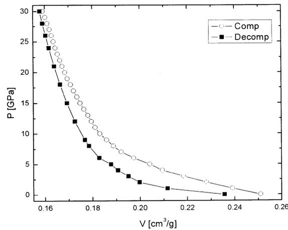
**Figure 8.** Variation of volume with pressure for vitreous GeO<sub>2</sub> at 300 K.
