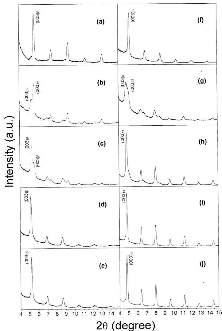
**Figure 5.** X-ray reflection patterns for (a) pure ZnA and mixed multilayers with (b) 2 mol% CdA, (c) 5 mol% CdA, (d) 10 mol% CdA, (e) 20 mol% CdA, (f) 25 mol% CdA, (g) 30 mol% CdA, (h) 50 mol% CdA, (i) 80 mol% CdA and (j) pure CdA (ref. [15]).
