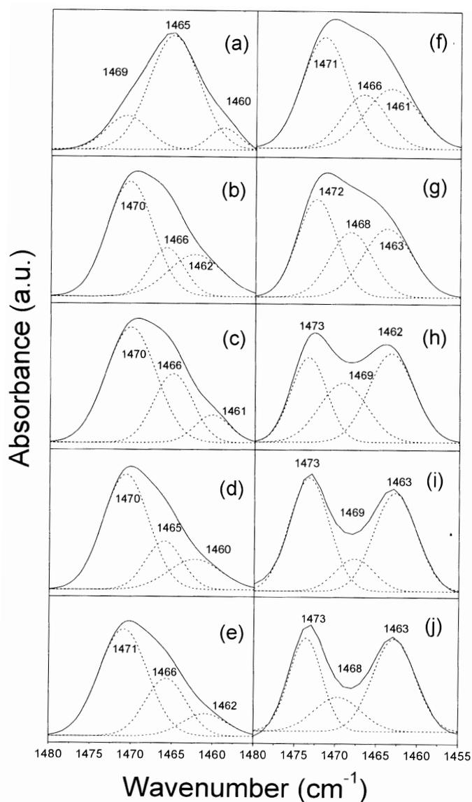
**Figure 4.** CH<sub>2</sub> scissoring band (*s*) for (a) pure ZnA and mixed multilayers with (b) 2 mol% CdA, (c) 5 mol% CdA, (d) 10 mol% CdA, (e) 20 mol% CdA, (f) 25 mol% CdA, (g) 30 mol% CdA, (h) 50 mol% CdA, (i) 80 mol% CdA and (j) pure CdA (ref. [15]).
