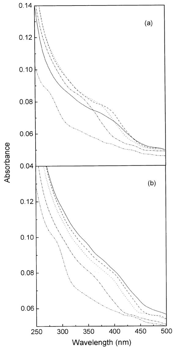
**Figure 8.** UV-Vis absorption spectra of the multilayers of pure CdA (—), mixed multilayers with 20 mol% ZnA (- - -), 50 mol% ZnA (···), 80 mol% ZnA (-·-·-) and pure ZnA (- - - -) after (a) 5 min and (b) 3 h H<sub>2</sub>S exposure (ref. [27]).
