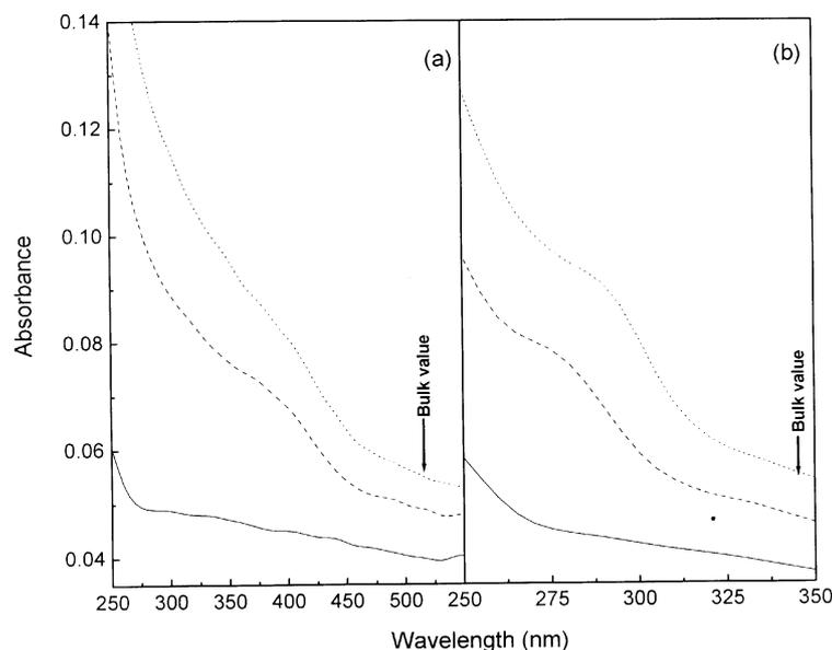
**Figure 7.** UV-Vis absorption spectra of (a) pure CdA multilayer and (b) pure ZnA multilayer in the as-deposited state (—) and after H<sub>2</sub>S exposed for 5 min (- - -) and 3 h (...). The enhanced absorption indicates the sulphide formation in the arachidic acid matrix. The bulk band gaps for CdS and ZnS are indicated (after ref. [27]).
