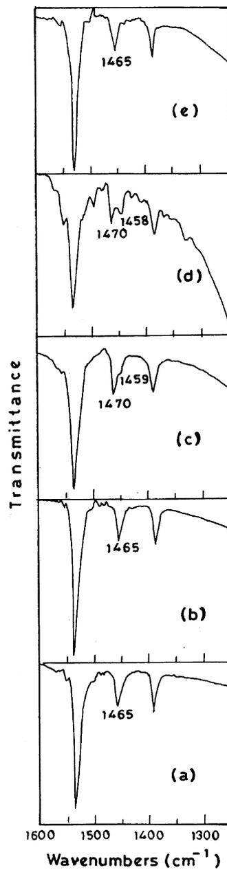
**Figure 3.** FTIR spectra of ZnA multilayers showing the CH<sub>2</sub> scissoring vibration of ZnA multilayers transferred at subphase pH values of (a) 6.5, (b) 6.8, (c) 7.3, (d) 7.4 and (e) 7.6, showing the nature of molecular packing in ZnA multilayers (ref. [30]).
