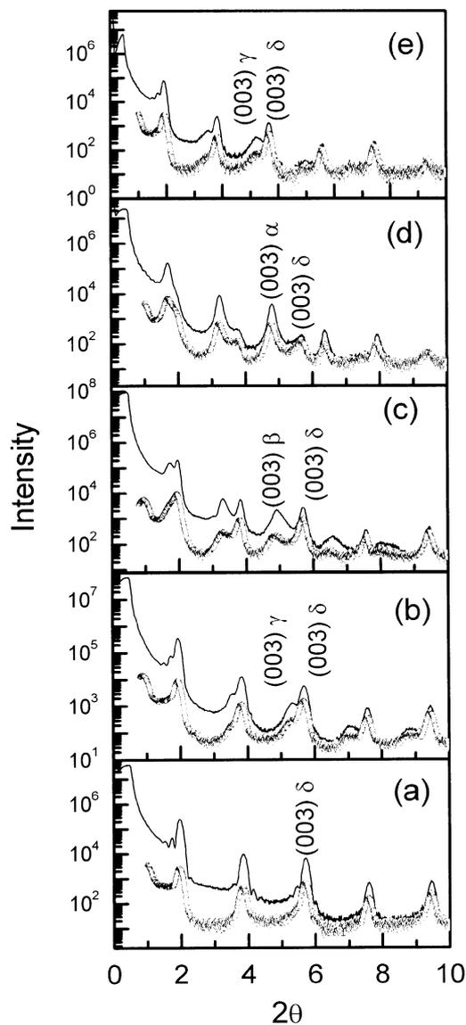
**Figure 1.** Longitudinal specular (solid line) and off-specular (open circles) scans for the ZnA multilayers transferred at subphase pH values of (a) 6.5, (b) 6.8, (c) 7.3, (d) 7.4 and (e) 7.6, showing the different types of layered structures present in ZnA multilayers (ref. [30]).
