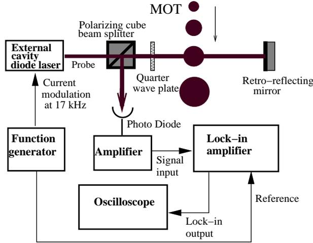
**Figure 1.** Schematic of the experimental set-up. The probe beam is 20 mm wide, which is more than the cloud size and 1 mm thick in the direction of gravity.
