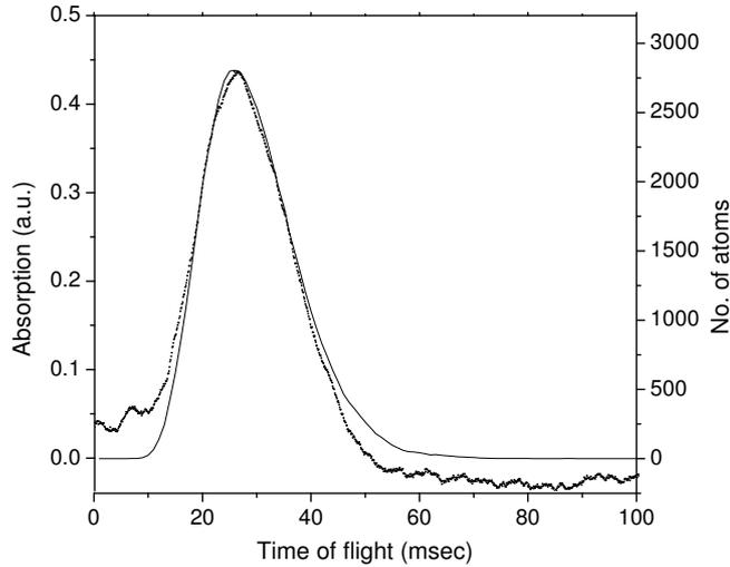
**Figure 4.** TOF signal of the atoms released from a MOT observed by keeping the probe beam 5 mm above the cloud. Dotted line is the TOF signal observed by the phase-sensitive probe absorption technique and it is averaged over 20 data. The probe power was  $5 \mu\text{W}$ . Solid line is the TOF signal obtained from the Monte Carlo simulation for a flat probe beam kept 5 mm above the MOT center.
