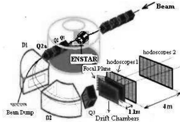
**Figure 1.** Experimental set-up for the proposed search of  $\eta$ -mesic nucleus at COSY by GEM Collaboration. The set-up uses Big Karl magnetic spectrometer (consisting of dipoles D1, D2 and quadrupoles Q1, Q2, Q2a and Q3), drift chambers and scintillator hodoscopes together with ENSTAR detector.
