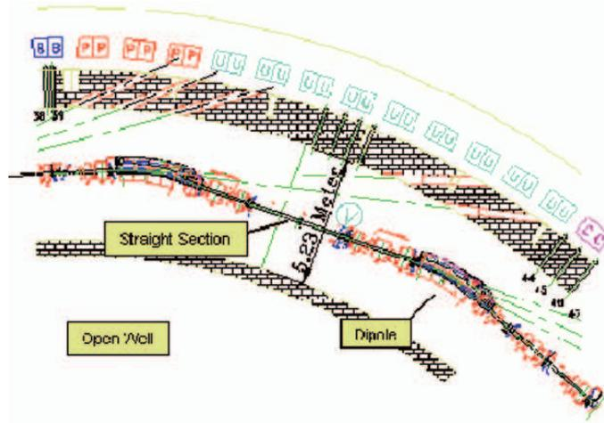
**Figure 10.** One of the straight sections in the Indus-2 beam line could be augmented for installation of the Laser Backscattered Photon facility. The dipole subsequent to the straight section would bend the electrons undergoing interaction with the laser photon for the purpose of tagging.
