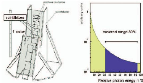
**Figure 6.** The tagger (left) at ELSA for tagging the electron. The  $1/E_\gamma$  spectrum of the bremsstrahlung photons is shown in the right panel. The shaded portion is the range covered with the SAPHIR detector. The tagging system was modified for the CB-TAPS system to have an energy range from 22 to 93% of the electron beam energy.
