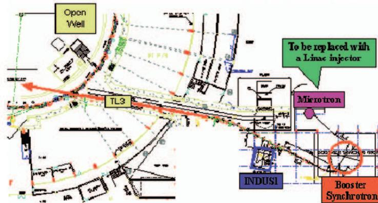
Figure 5. Actual lay-out of the 20 MeV Microtron Injector along with the Synchrotron Booster (700 MeV), Indus-1 (450 MeV Synchrotron) and part of the upcoming Indus-2 (2.5 GeV Synchrotron) at CAT, Indore, India. The transmission line TL3 meets the beam line of Indus-2 at the septum. The same TL3 can be extended into the ‘open well’ for bremsstrahlung studies.
