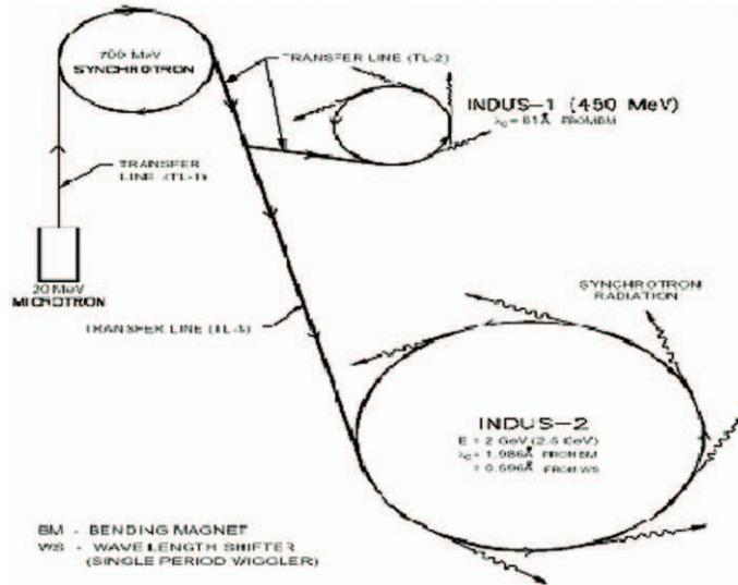
Figure 4. Schematic lay-out of the Microtron, Booster Synchrotron, Indus-1 and Indus-2 facility at CAT, Indore, India
