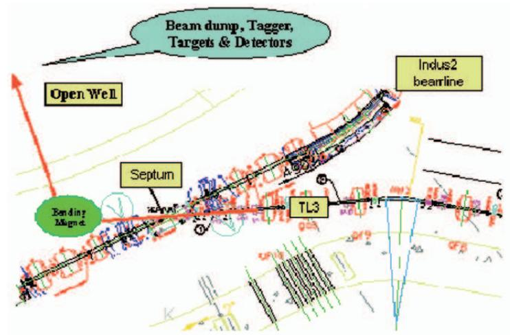
Figure 8. The TL3 beam line merging as an injector to Indus-2. The 700 MeV electron beam from the Synchrotron Booster can be suitably arranged to go straight forward and then bend into the open well for producing tagged bremsstrahlung photons.
