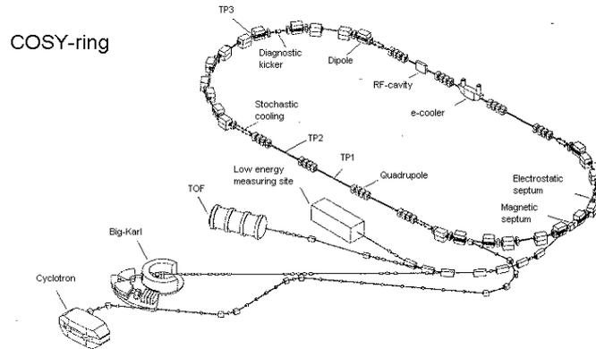
**Figure 1.** The floor plan of the COSY accelerator complex. JULIC is the injector cyclotron. The external target stations are the TOF (time-of-flight facility) and the Big Karl (magnetic spectrograph). The GEM experiments are done at the Big Karl area. In addition to external target stations several experiments are being done inside the ring which are not shown here.
