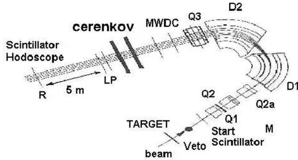
Figure 7. Experimental set-up for dibaryonic resonance search.
