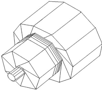
**Figure 2.** Perspective of one half of ENSTAR detector. Parts of the outer and middle layers are cut away to show the inner layers.
