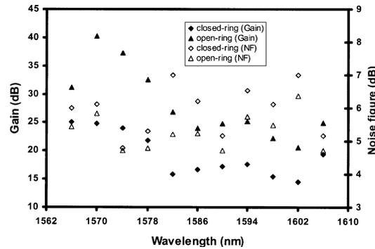
**Figure 3.** Gain and noise figure spectra for both amplifiers with open- and closed-ring.
