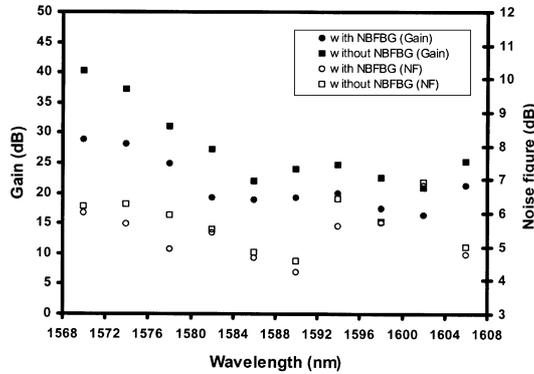
**Figure 6.** Gain and noise figure spectra for the gain-clamped amplifiers with and without NBFBG.
