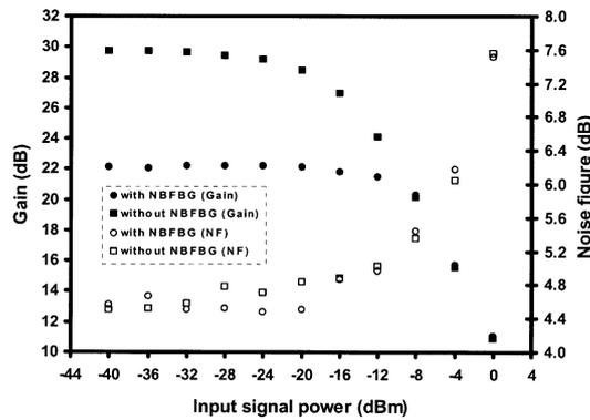
Figure 5. Gain and noise figure characteristics for the gain-clamped amplifier with NFBFG.
