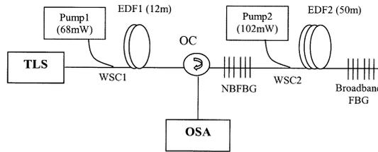
Figure 4. Gain-clamped double-pass L-band EDFA based on a partial reflection of ASE.
