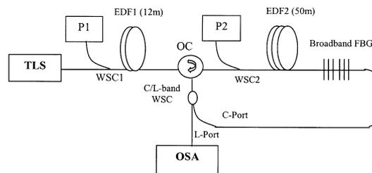
**Figure 1.** Gain-clamped double-pass L-band EDFA based on ring laser.
