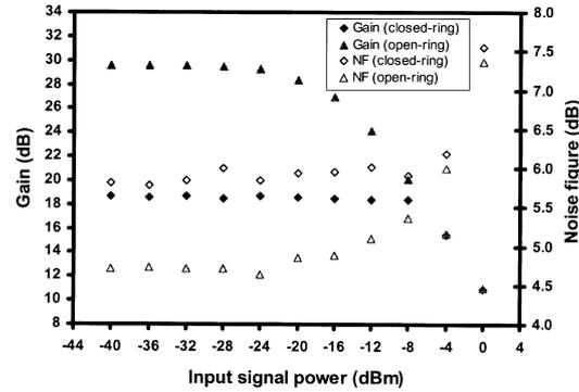
**Figure 2.** Gain and noise figure characteristics for the gain-clamped amplifier with ring laser.
