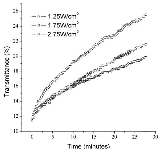
**Figure 5.** Measured transmittance of the erioglaucine dye-doped gelatin film as a function of time.
