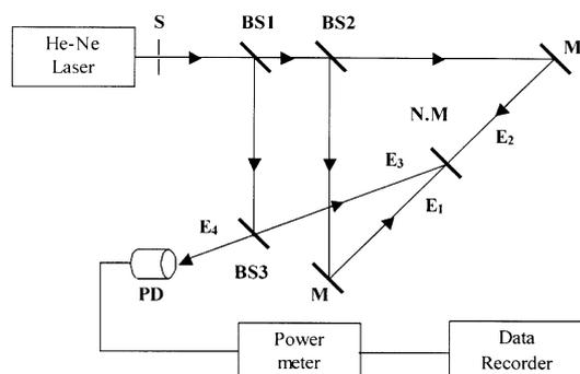
**Figure 3.** Experimental set-up for the observation of PC wave. S – shutter, BS1, BS2, BS3 – beam splitters, M – mirror, N.M – nonlinear medium, PD – photodetector.
