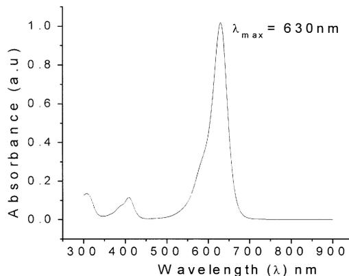
**Figure 2.** The UV-visible absorption spectra of erioglaucine dye.
