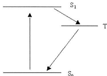
**Figure 4.** Schematic energy level diagram for erioglaucine dye saturable absorber.
