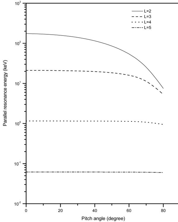
**Figure 2.** Variation of parallel resonance energy with pitch angle  $\alpha$  for  $L = 2, 3, 4$  and  $5$ .  $T_{\parallel} = 1200$  K and wave frequency  $\omega = 5$  kHz.
