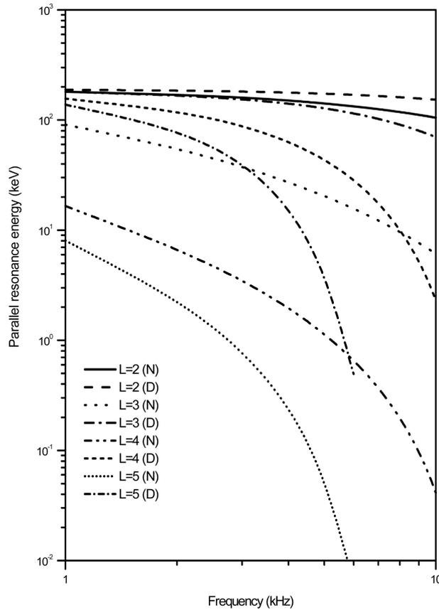
**Figure 1.** Variation of parallel resonance energy of electrons with wave frequency during normal (N) and disturbed (D) magnetospheric conditions for  $L = 2, 3, 4$  and  $5$ .  $T_{\parallel} = 1200$  K,  $A_T = 0.5$ , pitch angle  $\alpha = 30^\circ$ .
