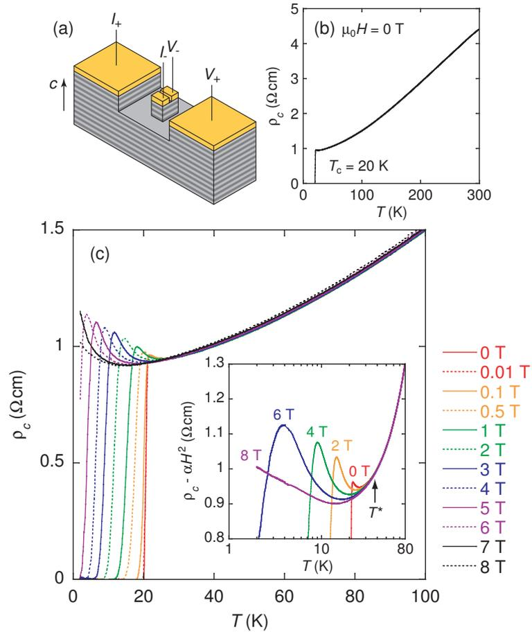
**Figure 1.** (a) Schematic illustration of our mesa structure (not to scale). (b) Temperature dependence of  $\rho_c$  in zero field for a mesa sample. (c)  $\rho_c(T)$  curves in magnetic fields applied along the  $c$ -axis. A slight field spread of the curves at high  $T$  is due to a small positive MR  $\propto H^2$ . After subtracting this MR all high- $T$  data follow a single curve (inset). Negative MR is observed below  $T^* \approx 38$  K.
