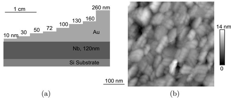
**Figure 1.** (a) Schematic cross-section of the full Nb–Au bilayer sample. (b) STM image ( $410 \times 410 \text{ nm}^2$ ) at 100 mK of the sample with a Au thickness of 72 nm. The rms roughness for this sample from this image is found to be 3.4 nm.
