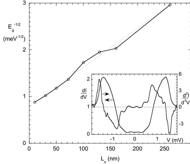
**Figure 3.** Variation of the quantity  $E_g^{-1/2}$ , the mini-gap  $E_g$  being defined in the inset by the inflection point in  $dI/dV(V)$ , with the N metal length  $L_n$ . The dashed line shows the best fit mini-gap as described by eq. (3). Inset: Tunneling spectra of the 50 nm sample together with its derivative  $d^2I/dV^2$ .
