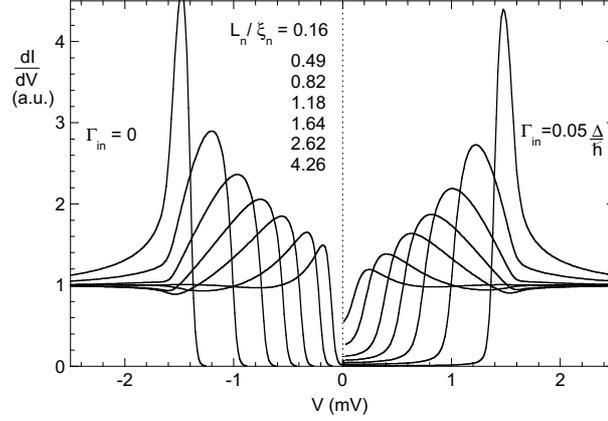
**Figure 4.** Calculated spectra using Usadel equations for a bilayer geometry with calculation parameters  $L_s/\xi_s = 5.17$ ,  $\Delta = 1.57$  meV,  $T = 210$  mK,  $\Gamma = 0.6$ ,  $r_B = 0$ , and  $\xi_n = 60.8$  nm. The right part ( $V < 0$ ) curve stands for  $\Gamma_{in} = 0$  and the left part ( $V > 0$ ) curve for  $\Gamma_{in} = 0.05\Delta/\hbar$ .
