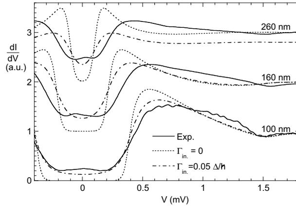
**Figure 5.** Comparison of the experimental data for  $L_n = 100, 160$  and  $260$  nm (full line) with the calculated spectra. The calculation parameters are  $L_s/\xi_s = 5.17$ ,  $\Delta = 1.57$  meV,  $T = 210$  mK,  $\Gamma = 0.6$ ,  $r_B = 0$ , and  $\xi_n = 60.8$  nm. The dotted line curve stands for  $\Gamma_{\text{in}} = 0$  and the dashed line curve for  $\Gamma_{\text{in}} = 0.05\Delta/\hbar$ . The curves have been evenly shifted for clarity.
