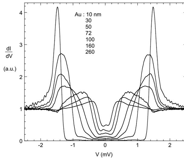
**Figure 2.** Tunneling density of states measured at 60 mK at the Au surface of Nb–Au bilayer samples with a varying Au thickness  $L_n$ . Data from the 130 and 200 nm samples are not shown for ease of reading.
