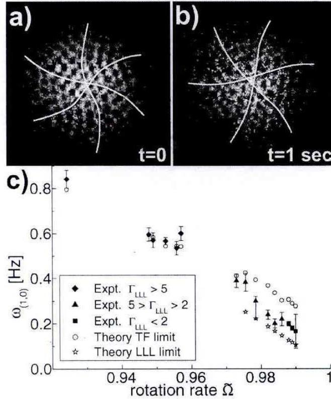
**Figure 13.** (a) and (b) show the Tkachenko mode at  $t = 0$  and at  $t = 1$  s for a condensate of  $1.5 \times 10^5$  atoms and  $\bar{\Omega} = 0.989$ . The mode has not even completed a quarter of its period of oscillation. (c) Comparison of Tkachenko mode frequency  $\omega_{1,0}$  (solid symbols) with theoretical predictions on the Thomas–Fermi limit (circles) and the quantum-Hall regime (stars). From ref. [43].
