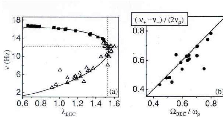
**Figure 5.** (a) Variation of the frequencies of the quadrupolar modes as a function of the aspect ratio. The continuous curve is the best fit from theory. (b) Frequency splitting of the quadrupolar modes as a function of  $\Omega/\omega_{\perp}$  obtained from the aspect ratio  $\lambda$  using eq. (5.6).
