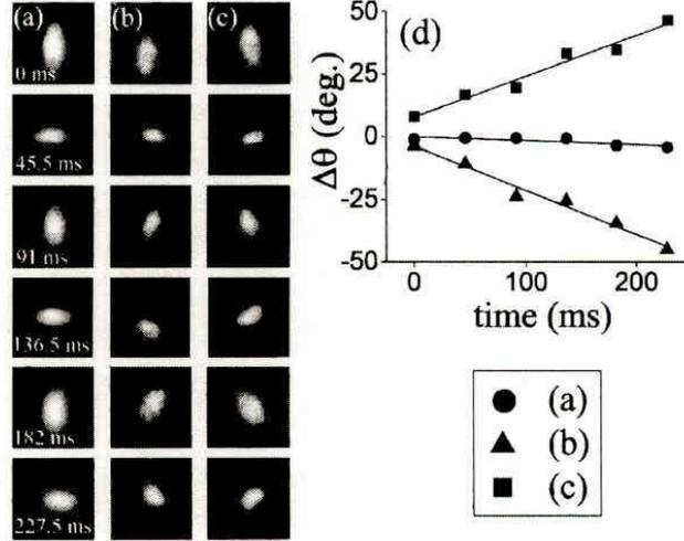
**Figure 4.** Quadrupolar modes excited in (a) a vortex free condensate of  $^{87}\text{Rb}$ , (b) and (c) are quadrupolar modes in a condensate with a vortex. The images are non-destructive and strobed at intervals of 45.5 ms. The trap frequency  $\nu_{\perp} = 7.8$  Hz [16]. The linear fit to the angle of rotation as a function yields a value  $-0.49(4)$  Hz for the precession frequency in (b) and  $0.45(5)$  Hz for the precession frequency in (c).
