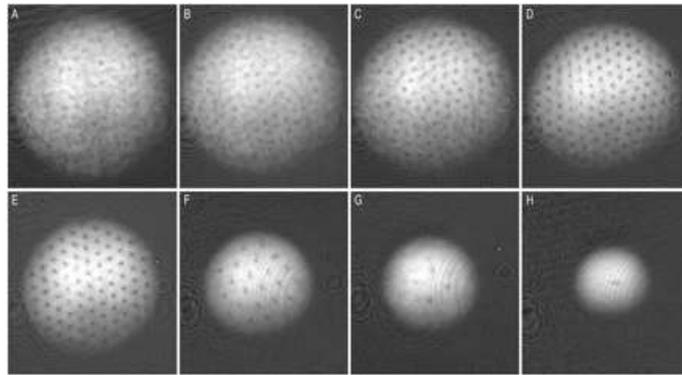
**Figure 8.** Growth and decay of the vortex lattice when a condensate of  $^{23}\text{Na}$  was rotated in an axially symmetric trap and held in the trap for different times after the rotating laser beams were switched off. (A) 25 ms; (B) 100 ms; (C) 200 ms; (D) 500 ms; (E) 1 s; (F) 5 s; (G) 10 s and (H) 40 s. The temperature was below the condensation temperature such that 90% of the atoms were in the condensate. From ref. [14].
