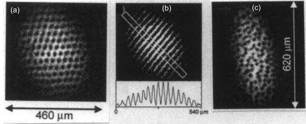
**Figure 10.** Rotating condensate (a) with a perfect vortex lattice arrangement when no quadrupolar surface mode is excited; (b) sheet-like structures due to merging of vortex cores along the minor axis of the condensate when the quadrupolar surface mode  $\ell = 2$ ,  $m_\ell = -2$  is excited and; (c) irregular distribution of vortices when the surface mode  $\ell = 2$ ,  $m_\ell = +2$  is excited. From ref. [34].
