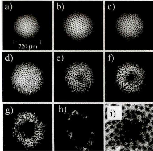
**Figure 15.** Stages in the formation of a giant vortex. Starting point is (a) with a condensate of  $^{87}\text{Rb}$  with 180 vortices. Atoms are removed from near the axis by shining a 8 fW power for (b) 14 s. We now have 250 vortices due to decrease in the number of atoms. (c) 15 s, (d) 20 s, (e) 22 s, (f) 23 s, (g) = 40 s and (h) 70 s when light is on. (i) is a close-up picture of the core region in (f). From ref. [46].
