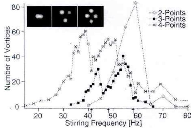
**Figure 7.** Number of vortices in the condensate as a function of frequency for two- (○) three- (●) and four- (×) stirring with a laser beam of waist  $25 \mu\text{m}$  [27]. Arrows indicate the values of  $\omega_\ell/\ell$  for  $\ell = 2, 3$  and  $4$ .
