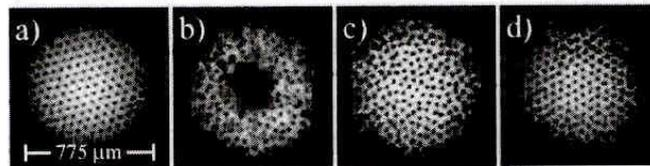
**Figure 16.** Lattice reforming after giant vortex formation. (a) The starting vortex lattice, (b) after a pulse of 60 fW for 2.5 s of the atom blasting laser. The hold time in the trap after the pulse is (c) 10 s and (d) 20 s.
