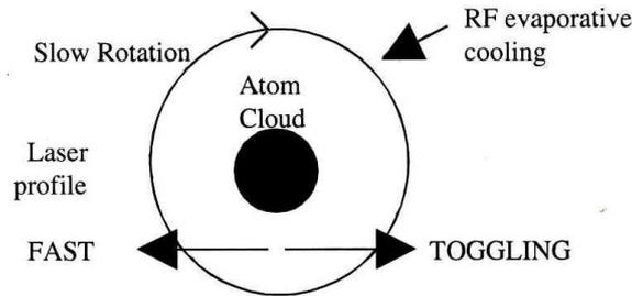
**Figure 3.** Rotation of the vapour of  $^{87}\text{Rb}$  as it is cooled in an Ioffe–Pritchard trap. The plane shown is perpendicular to the axis of the Ioffe–Pritchard trap. Far-detuned laser beam travelling parallel to the axis and focussed  $8 \mu\text{m}$  away from the axis is toggled at 100 kHz from right to left. At the same time the laser spot is rotated slowly at the rate  $\Omega$  about the axis. The cloud is cooled by RF evaporative cooling to below  $T_c$ .
