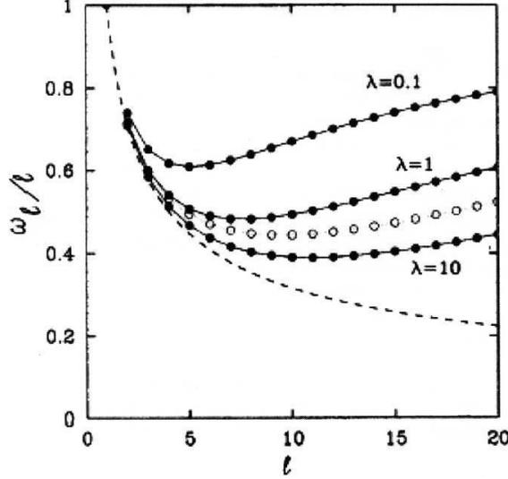
**Figure 6.** The quantity  $\omega_\ell/\ell$  in units of  $\omega_\perp$  as a function of  $\ell$  for a condensate of  $^{87}\text{Rb}$  for three trap aspect ratios  $\lambda = \omega_z/\omega_\perp$ . The total number of atoms  $N = 10^5$  and the geometric mean frequency  $\bar{\omega}$  is 20 Hz. These results are obtained from the sum rule. Open circles represent exact solutions of Bogulibov's equation. Dashed line is the hydrodynamic prediction  $\omega_\ell/\ell = 1/\sqrt{\ell}$ .
