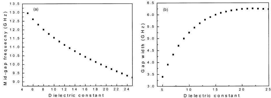
**Figure 3.** (a) The variation in the mid-gap frequency with dielectric constant. The lattice spacing was chosen as 1.0 cm and the radius of the sample was taken as 0.207 cm. (b) The variation in the gap width with dielectric constant. The lattice spacing was chosen as 1.0 cm and the radius of the sample was taken as 0.207 cm.
