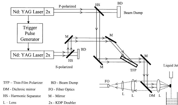
**Figure 1.** Schematic diagram for recording LIBS under double laser pulse excitation as well as the ray diagram for making two synchronized lasers collinear.
