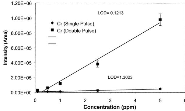
**Figure 3.** Variation in emission (425.44 nm) from chromium with concentration under single [laser = 140 mJ, gate delay/gate width = 20  $\mu$ s/10  $\mu$ s] and double pulse excitation [laser (1) = 140 mJ, laser (2) = 140 mJ, gate delay (from first laser)/gate width = 20  $\mu$ s /10  $\mu$ s, delay between lasers = 2.5  $\mu$ s].
