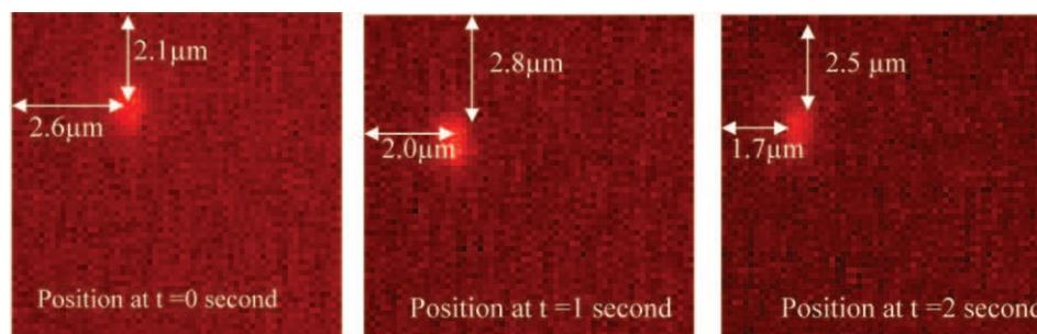
**Figure 3.** Sequential images ( $1000 \times$  magnification) of *in-vitro* assay at 1 s interval. The fluorescent spot is the actin filament moving on myosin track. The figure indicates the changing position of the actin filament at different time intervals.
