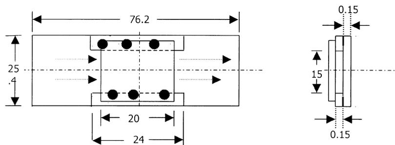
**Figure 1.** Flow cell prepared from coverslip and glass slide. The arrows show the inflow and outflow of the buffer solution during motility assay. (Note: All dimensions are in mm.)
