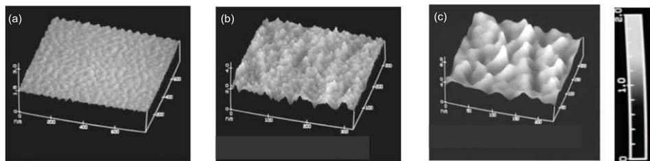
**Figure 2.** Contact mode AFM images of myosin cross-linked to lysine-coated glass slide. (a) Glass slide coated with lysine (roughness 0.5 nm), (b) EDC-coated on lysine-coated glass slide (roughness 1.2–1.4 nm), (c) myosin molecules immobilized with EDC (roughness 2.4–4.5 nm).
