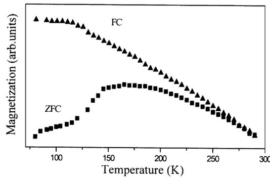
**Figure 7.** The zero-field cooled and field-cooled magnetization for the 25 nm particles of  $\text{Mn}_{0.67}\text{Zn}_{0.33}\text{Fe}_2\text{O}_4$ .
