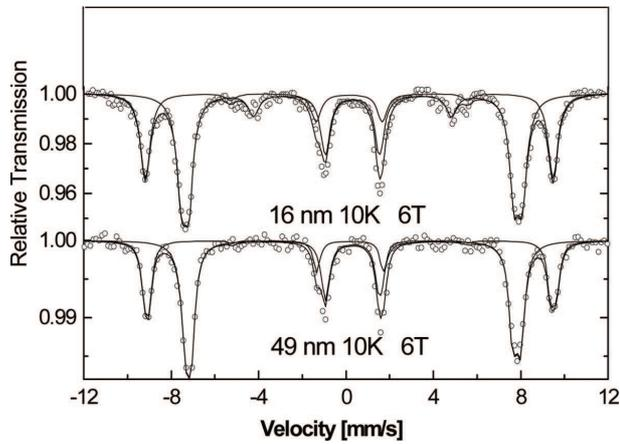
**Figure 3.** The Mössbauer spectra in an external magnetic field of 6 T applied parallel to the  $\gamma$ -ray direction for the unmilled and 15 h milled  $\text{Ni}_{0.5}\text{Zn}_{0.5}\text{Fe}_2\text{O}_4$  samples.
