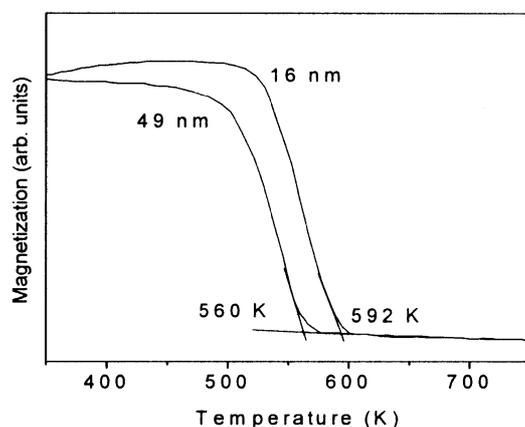
**Figure 2.** The thermogravimetric plot for the nanostructured  $\text{Ni}_{0.5}\text{Zn}_{0.5}\text{Fe}_2\text{O}_4$  with average grain sizes 49 nm and 16 nm.
