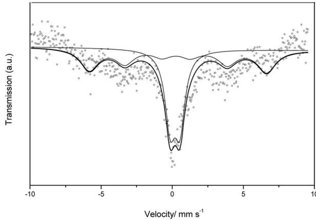
**Figure 6.** The Mössbauer spectrum at 300 K of the 25 nm particles of  $\text{Mn}_{0.67}\text{Zn}_{0.33}\text{Fe}_2\text{O}_4$ .
