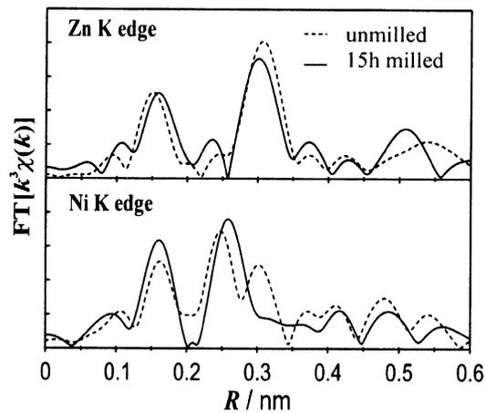
**Figure 4.** The Fourier-transform of the EXAFS spectrum of the unmilled and the 15 h milled  $\text{Ni}_{0.5}\text{Zn}_{0.5}\text{Fe}_2\text{O}_4$  samples for Zn and Ni K edges.
