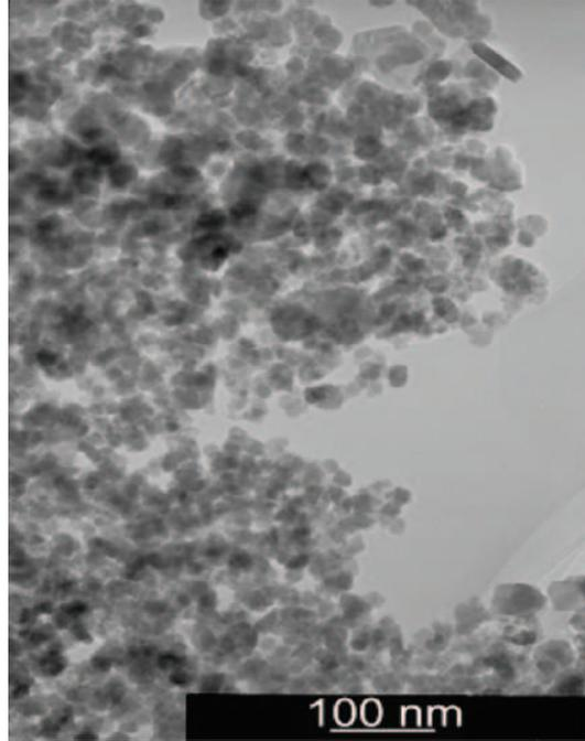
**Figure 5.** The TEM picture of the 25 nm particles of  $\text{Mn}_{0.67}\text{Zn}_{0.33}\text{Fe}_2\text{O}_4$  sample.
