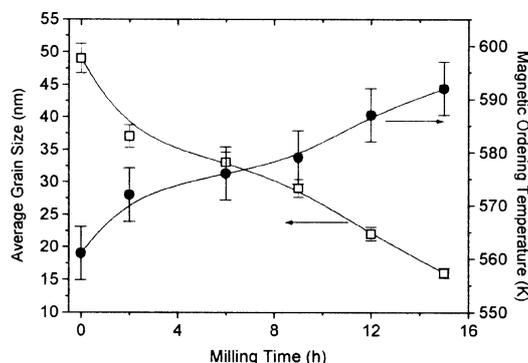
**Figure 1.** The variation of the average grain size and the magnetic ordering temperature of nanostructured  $\text{Ni}_{0.5}\text{Zn}_{0.5}\text{Fe}_2\text{O}_4$  as a function of milling time.
