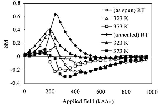
**Figure 8.** The  $\delta M$  plot of the as-spun and annealed  $\text{Nd}_{10}\text{Fe}_{85}\text{B}_5$  ribbons at 293 K, 323 K and 373 K (open symbols represent the as-spun ribbons and the filled ones represent annealed ribbons).
