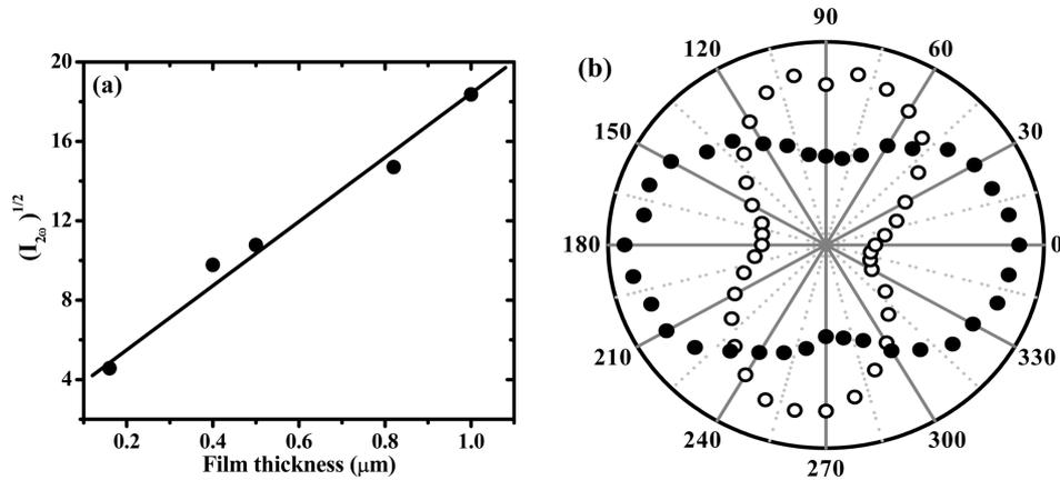
**Figure 5.** (a) Dependence of the SHG of ZNDA film on the thickness; (b) polar plots of the SHG in q-p ( $\bullet$ ) and q-s ( $\circ$ ) geometries as a function of the angle of rotation of the plane of polarization of the fundamental wave; the zero of the scale is chosen to coincide with one of the maxima in the q-p geometry.
