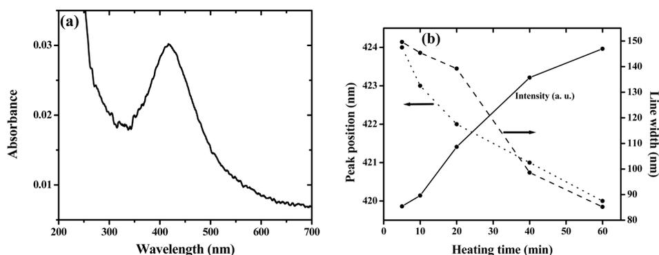
**Figure 6.** (a) Electronic absorption spectrum of Ag-PVA film (Ag/PVA = 0.042, thermal treatment time, temperature = 60 min, 90°C). (b) Variation of the intensity, peak maximum and peak width of the absorption of the Ag-PVA film with the time of thermal treatment.
