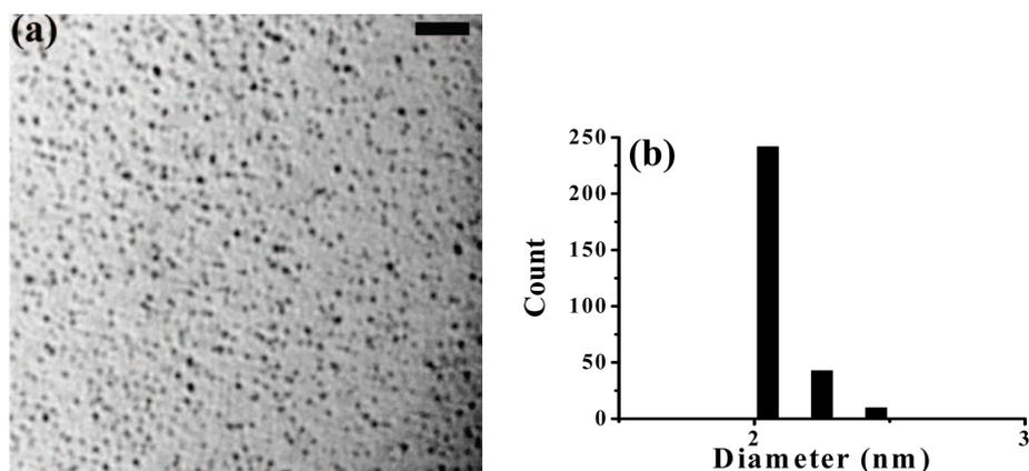
**Figure 7.** (a) TEM image of Ag-PVA film (Ag/PVA = 0.042, thermal treatment time, temperature = 60 min, 110°C). Scale bar = 20 nm. (b) Histogram of the particle size distribution in the image shown in (a).
