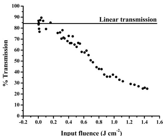
**Figure 8.** Optical limiting in Ag-PVA/PS film (Ag/PVA = 0.058, thermal treatment time, temperature = 60 min, 90°C) at 532 nm.
