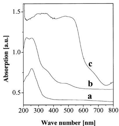
**Figure 4.** UV-visible diffuse reflectance spectra of surfactant free Fe-MCM-41 (curve a), Fe<sub>2</sub>O<sub>3</sub> embedded mesoporous silica (curve b, sample 2) and bulk Fe<sub>2</sub>O<sub>3</sub> (curve c).
