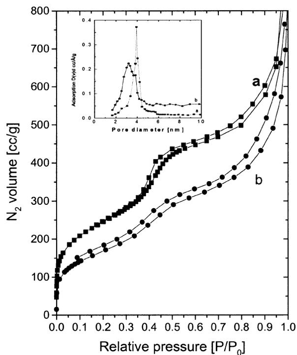
**Figure 3.** N<sub>2</sub> adsorption/desorption isotherms of mesoporous MCM-41 (curve a) and sample 2 (curve b) after iron loading. BJH pore size distributions are shown in the inset.
