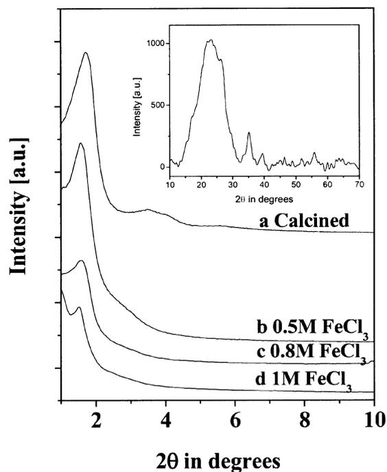
**Figure 1.** XRD patterns of mesoporous support MCM-41 (curve a, sample 1) before iron loading and Fe<sub>2</sub>O<sub>3</sub> embedded mesoporous silica samples 2 (curve b, 0.5 M FeCl<sub>3</sub>), 3 (curve c, 0.8 M FeCl<sub>3</sub>) and 4 (curve d, 1 M 0.5 M FeCl<sub>3</sub>). High angle diffraction pattern of sample 2 is shown in the inset.
