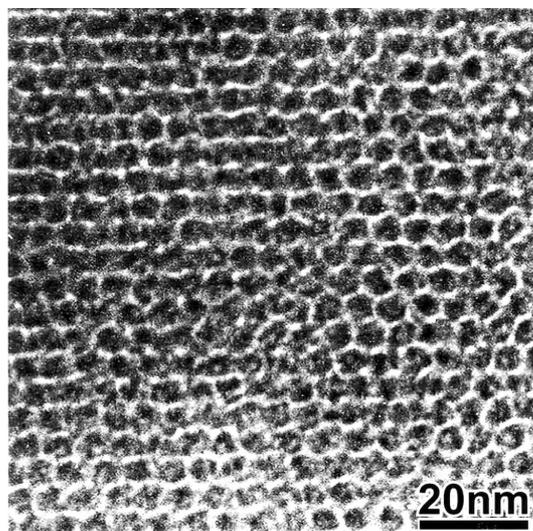
**Figure 2.** TEM image of  $\text{Fe}_2\text{O}_3$  nanoparticles in the mesoporous silica (sample 2).
