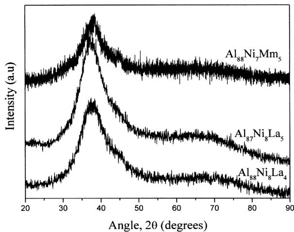
**Figure 2.** XRD patterns of as-melt-spun Al–Ni–RE amorphous ribbons on the air-cooled side.
