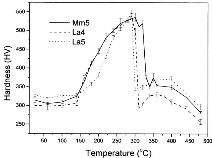
**Figure 4.** Isochronal microhardness evolution of different Al-Ni-RE ribbons. The samples were annealed for 10 min at each measuring temperature.
