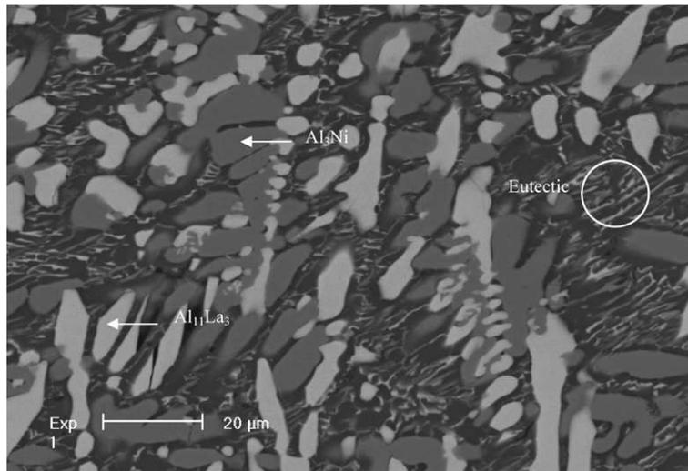
**Figure 1.** SEM back-scattered image of Al<sub>87</sub>Ni<sub>8</sub>La<sub>5</sub> ingot, the phases are marked.
