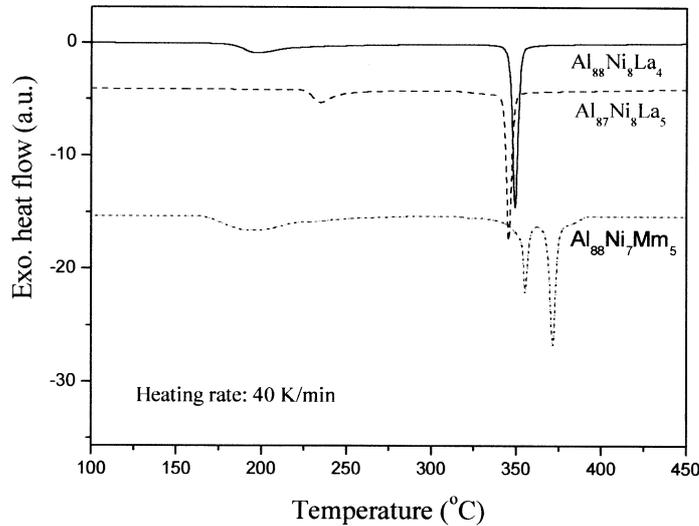
**Figure 3.** DSC curves of amorphous Al-Ni-RE (RE = La/Mm) alloys at a heating rate of 40 K/min.
