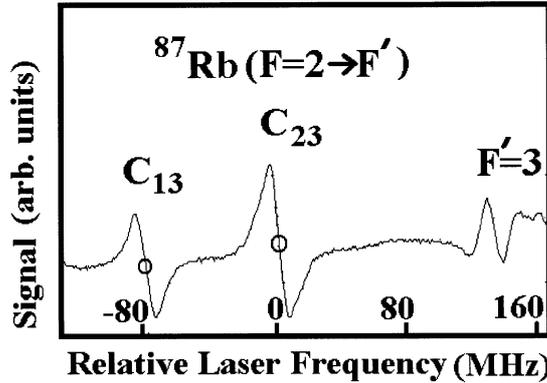
**Figure 2.** Oscilloscope trace of the DFDL signal. The circles denote frequencies at which the two diode lasers were locked. The applied magnetic field was 10 G.
