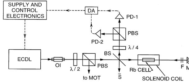
**Figure 1.** Schematic of the experimental set-up for frequency stabilization using Doppler-free dichroic lock. ECDL: External cavity diode laser; MOT: magneto-optical trap; BS: beam splitter plate; S: stopper; PBS: polarizing cube beam splitter; F: neutral density filters; M: mirror, OI: optical isolator; PD: photodiode; DA: difference amplifier.
