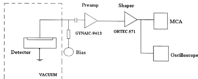
Figure 4. Block diagram of measurement set-up for  $\alpha$ -particle spectroscopy.
