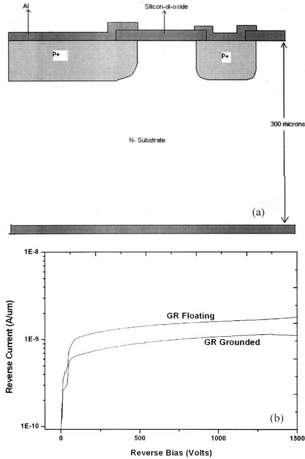
**Figure 7.** (a) Device structure for MEDICI simulations. (b)  $I$ - $V$  characteristics of the simulated device under different biasing conditions of the guard ring.
