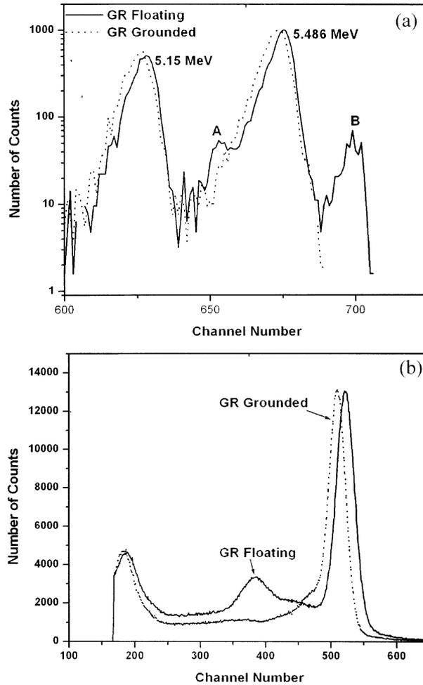
**Figure 6.** (a) Count vs. energy showing a typical  $\gamma$ -ray (60 keV) spectrum under two conditions of guard ring floating and grounded. (b) Count vs. channel number showing  $\alpha$ -particle spectra for  $^{241}\text{Am}$  and  $^{239}\text{Pu}$  under the conditions of guard ring floating or grounded, spurious peaks disappear after biasing the guard ring.
