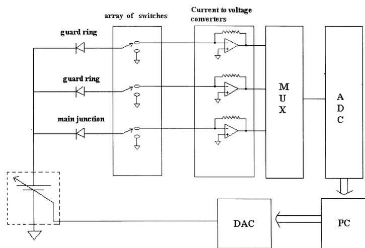
**Figure 2.** Schematic circuit diagram of the set-up used for the characterization of silicon detectors.
