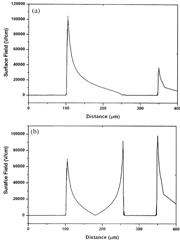
**Figure 9.** Surface field along the lateral dimension of the simulated structure at reverse bias of 500 V under the condition that guard ring is (a) floating or (b) biased.
