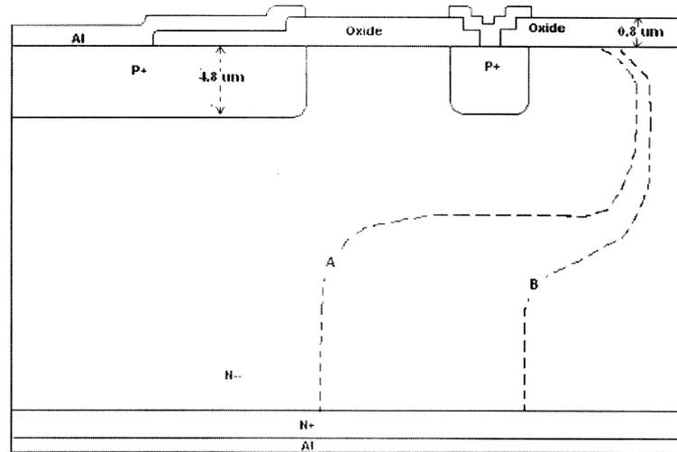
**Figure 10.** Depletion edges on the periphery of the detector under two conditions of guard ring floating (edge A) and grounded (edge B) and more than full depletion voltage applied at backside ohmic contact.
