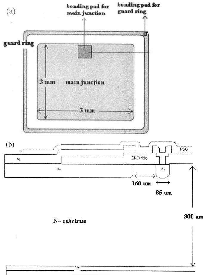
**Figure 5.** (a) Top view and (b) cross-sectional view of the 36 mm<sup>2</sup> diode used for  $\alpha$ -spectroscopy.
