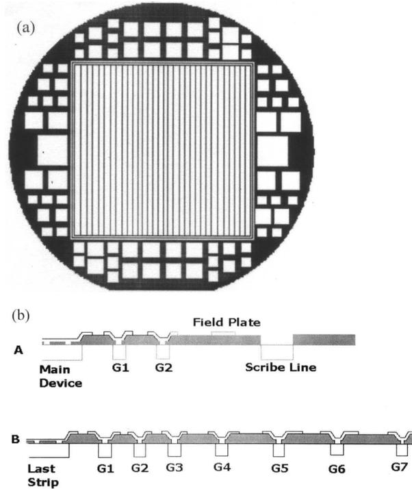
**Figure 1.** (a) Fabricated 4" wafer showing strip detector of area  $6.3 \times 6.3 \text{ cm}^2$  and other small area detectors. (b) Schematic cross-section of diode detector and strip detector.
