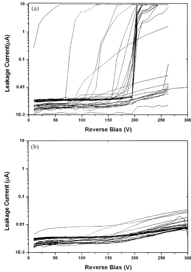
Figure 3.  $I$ - $V$  characteristics of a 32-strip detector under the conditions of (a) guard ring floating and (b) guard ring biased.
