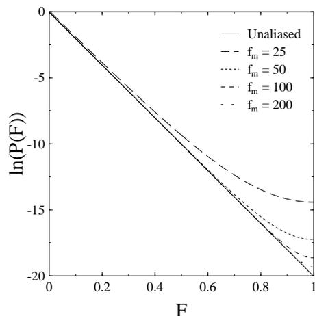
**Figure 1.** Aliased exponential decay of sampled data with different Nyquist frequencies. As  $f_m$  increases, the power spectrum tends to the true one.
