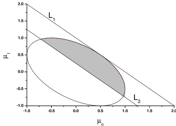
**Figure 7.** Phase diagram for the ternary sequence.  $L_1$  and  $L_2$  label the lines  $\mu_0 + \mu_1 = 1$  and  $\mu_0 + \mu_1 = \frac{1}{4}$ , respectively. The regions inside and outside the ellipse correspond to the diffusive and super-diffusive regimes, respectively. The shaded region, though diffusive for the ternary sequence, is super-diffusive when the ternary sequence is coarse-grained into a binary sequence.
