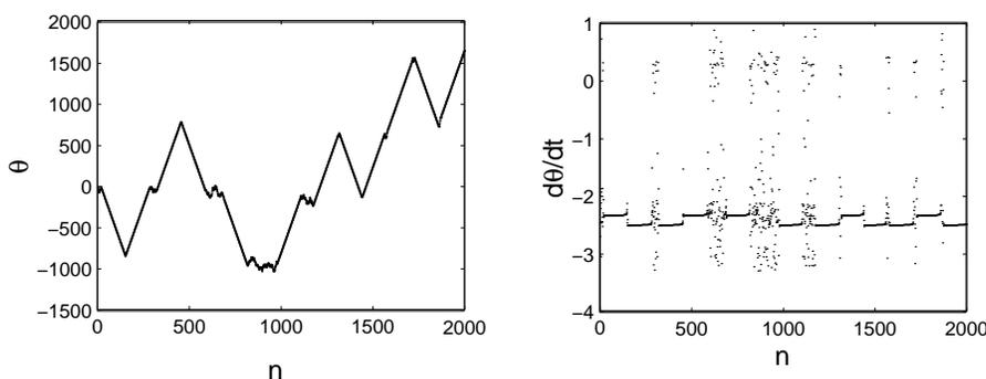
**Figure 6.**  $\theta$  (left) and  $\dot{\theta}$  (right) as functions of the Strobe time  $n$  for the driven, damped pendulum.
