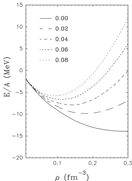
**Figure 1.** EOS of symmetric nuclear matter when  $\sigma$ -nucleon coupling constant of Bonn potential is modified according to eq. (1). Various curves correspond to different values of  $\alpha$  of eq. (1).
