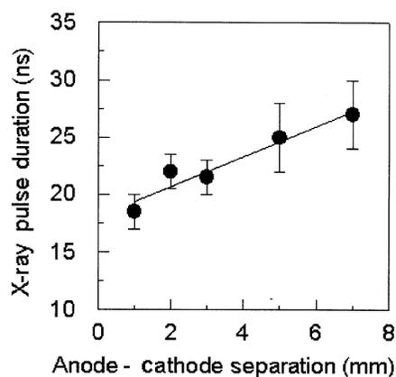
Figure 2. Dependence of the  $K_{\alpha}$  x-ray pulse duration on the anode-cathode separation (laser energy = 25 mJ, anode voltage = 20 kV).
