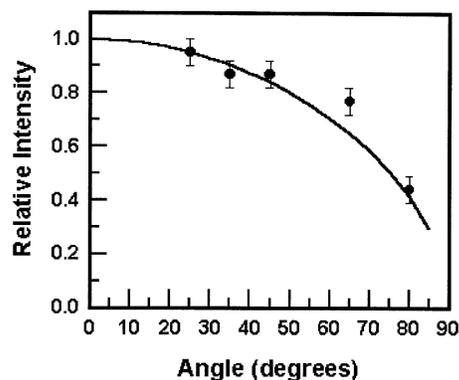
**Figure 5.** Angular distribution of the x-ray emission from the anode tip. The solid curve represents a  $\cos^{0.5} \theta$  distribution.
