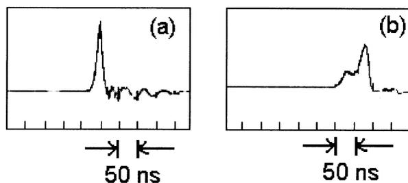
**Figure 3.** Typical temporal profiles of  $K_\alpha$  x-ray emission. (a)  $d = 2$  mm, (b)  $d = 10$  mm.
