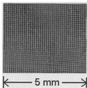
**Figure 6.** Single-shot x-ray radiograph of a copper wire mesh recorded using the  $K_{\alpha}$  x-ray source. The wire thickness and grid separation of the wire mesh is  $\sim 60$   $\mu\text{m}$  each.
