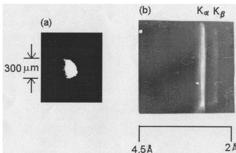
**Figure 4.** (a) Spatial profile of the  $K_\alpha$  x-ray source, (b) x-ray emission spectrum from titanium anode.  $K_\alpha$ : 4.51 keV (2.75  $\text{\AA}$ ),  $K_\beta$ : 4.93 keV (2.51  $\text{\AA}$ ).
