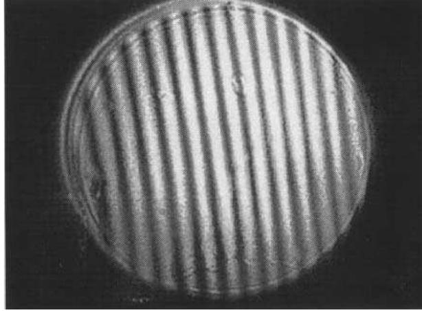
**Figure 4.** Photograph of a typical finite-fringe interferogram.
