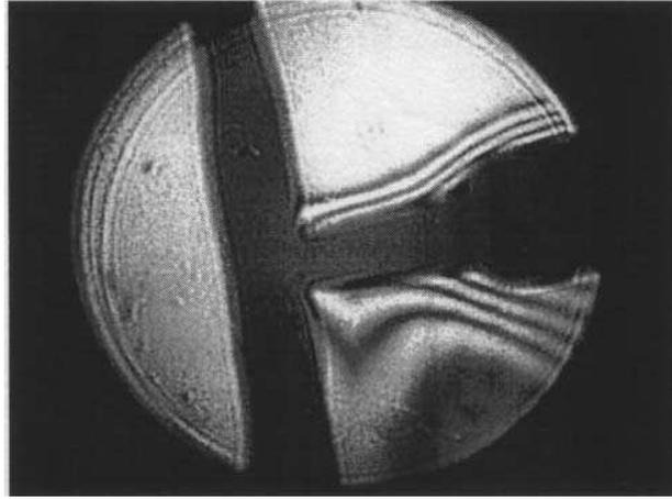
**Figure 6.** Photograph of typical interference pattern of heat flow obtained by inserting a hot soldering gun with a vertical metallic sheet in the test arm.
