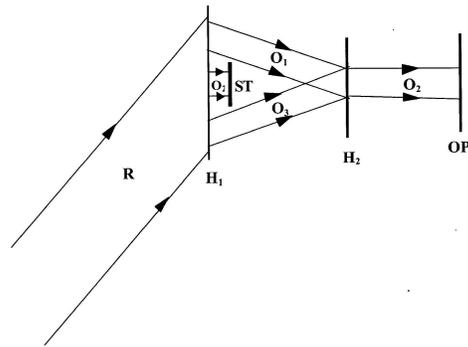
**Figure 3.** Schematic configuration for forming holographic optics-based interferometer.
