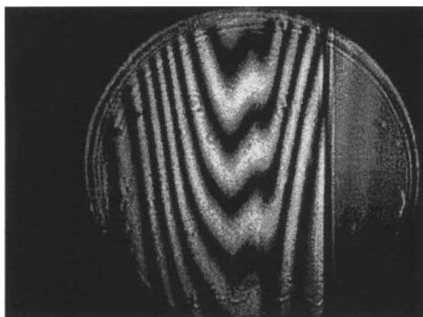
**Figure 8.** Photograph of interference pattern obtained by inserting a microscope cover slide plate in the test arm.
