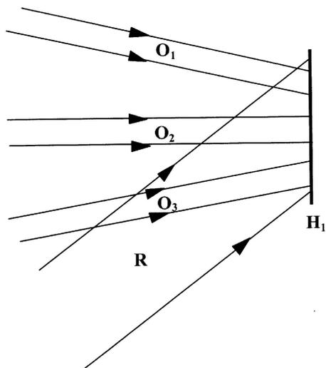
**Figure 1.** Recording scheme for the generation of holographic optical elements on plate  $H_1$ .
