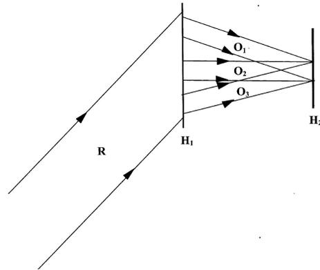
**Figure 2.** Recording scheme for the generation of holographic optical elements on plate  $H_2$ .
