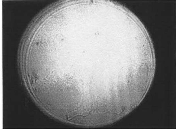
**Figure 5.** Photograph of a typical infinite-fringe interferogram.
