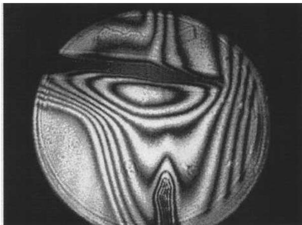
**Figure 7.** Photograph of typical interference pattern of heat flow obtained by inserting a metallic sheet over a burning candle in the test arm.
