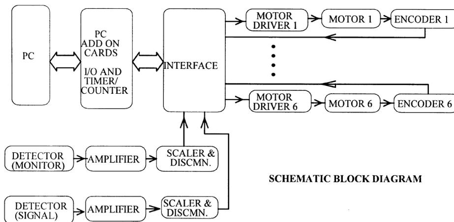
**Figure 1.** Schematic block diagram of data acquisition and instrument control system.
