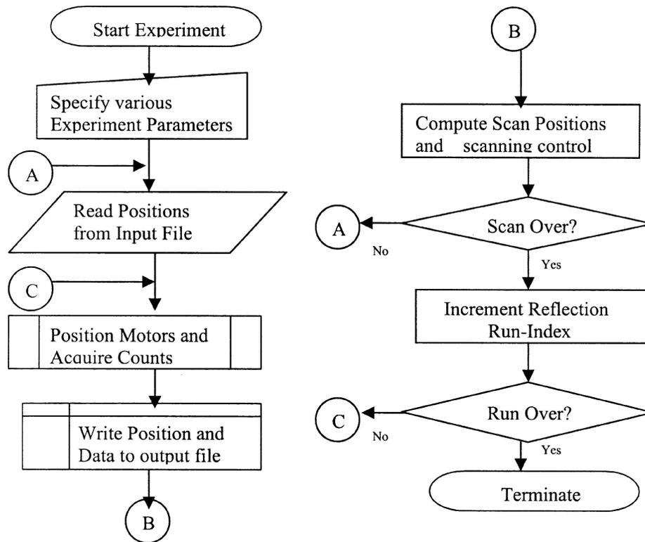
Figure 2. Flow chart of a scan.
