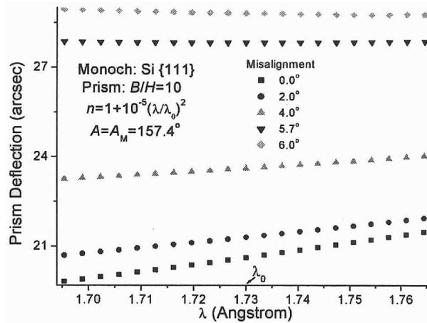
Figure 5. Minimising  $\delta$  variation by misaligning isosceles prism.
