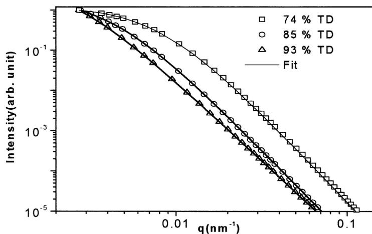
Figure 4. Fit of the model to the extracted single scattering profiles for three sintering.
