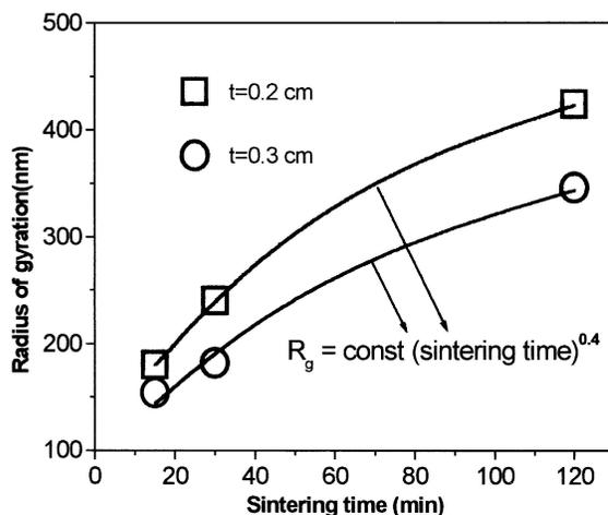
Figure 3. The evolution of the radius of gyration with sintering time.
