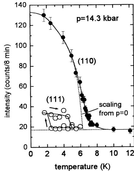
**Figure 1.** Temperature dependence of the magnetic scattering intensity observed in the (110) and (111) directions, respectively, at a pressure slightly below the critical pressure  $p_c$ .
