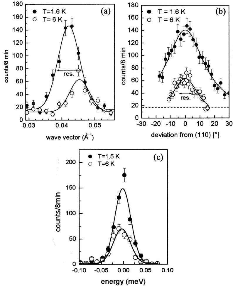
**Figure 2.** Neutron scattering scans through the magnetic Bragg peaks in the (110) direction at  $p = 14.3$  kbar in the longitudinal direction (a) and in the transverse direction (b) as well as in energy (c).
