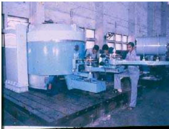
**Figure 1.** Prototype triple-axis spectrometer under test.
