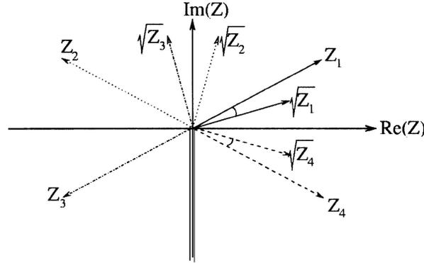
**Figure 1.** The Argand diagram for the complex wave-vectors  $k_z = \sqrt{Z}$  for the four cases of absorption and amplification of propagating or evanescent waves. The branch cut in the complex plane is shown along the negative imaginary axis.
