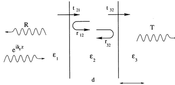
**Figure 2.** Schematic for transmission through a dielectric amplifying or absorbing slab. The notation for the partial reflection and transmission (Fresnel) coefficients are indicated.
