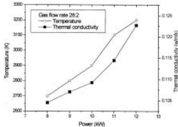
**Figure 12.** Variation of temperature and thermal conductivity with increase in input power at a total gas flow rate of 30 lpm.
