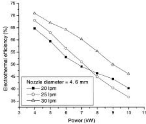
Figure 2. Variation of electrothermal efficiency with increase in input power at various argon gas flow rates.
