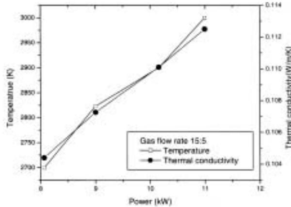
**Figure 10.** Variation of temperature and thermal conductivity with increase in input power at a total gas flow rate of 20 lpm.
