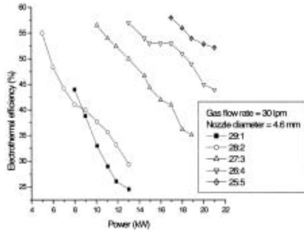
**Figure 5.** Variation of electrothermal efficiency with increase in input power at a nitrogen mixture gas flow rate of 30 lpm.
