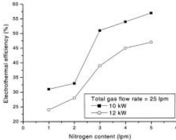
**Figure 7.** Variation of electrothermal efficiency with increase in nitrogen content at two input power levels. Total gas flow rate is 25 lpm.
