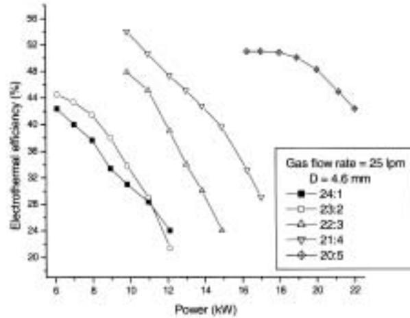
**Figure 4.** Variation of electrothermal efficiency with increase in input power at a nitrogen mixture gas flow rate of 25 lpm.
