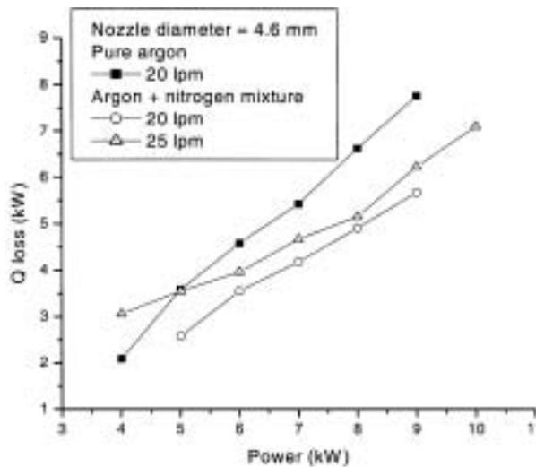
**Figure 9.** Dependence of  $Q$  loss in input power.
