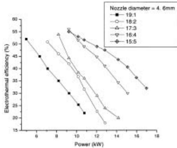
Figure 3. Variation of electrothermal efficiency with increase in input power at various nitrogen mixture gas flow rates.
