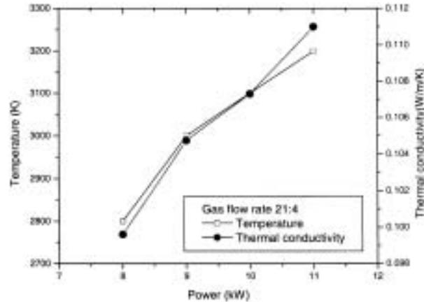
**Figure 11.** Variation of temperature and thermal conductivity with increase in input power at a total gas flow rate of 25 lpm.
