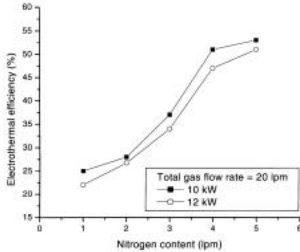
**Figure 6.** Variation of electrothermal efficiency with increase in nitrogen content at two input power levels. Total gas flow rate is 20 lpm.
