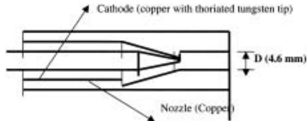
Figure 1. Schematic of a DC plasma spray torch.
