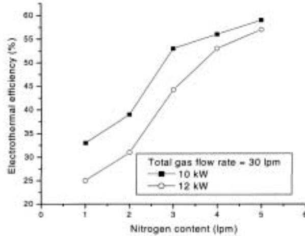
**Figure 8.** Variation of electrothermal efficiency with increase in nitrogen content at two input power levels. Total gas flow rate is 30 lpm.
