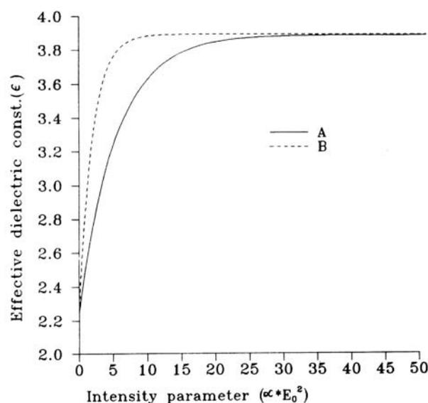
**Figure 1.** Variation of the effective dielectric constant ( $\epsilon$ ) with the electric field intensity parameter ( $\alpha E_0^2$ ) for Kerr non-linearity. Curve A denotes the present analysis and Curve B the paraxial ray approximation method. Here  $\epsilon_{CO} = 2.25$ ,  $\epsilon_S = 0.73$ ,  $r_0 = 25 \mu\text{m}$  and  $a_0 = 25 \mu\text{m}$ .
