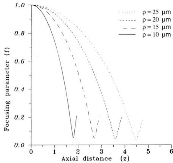
**Figure 6.** Plot of beam width parameter ( $f$ ) with axial distance ( $z$ ) for the saturating Kerr non-linearity in the case of parabolic fiber for different values of transverse distance ( $\rho$ ) from the axis of fiber.  $\epsilon_S = 0.01125$ ,  $E_0 = 1 \times 10^{10}$ ,  $\lambda = 1.55 \mu\text{m}$ ,  $\Delta = 0.001$ ,  $r_0 = 25 \mu\text{m}$  and  $a_0 = 25 \mu\text{m}$ .
