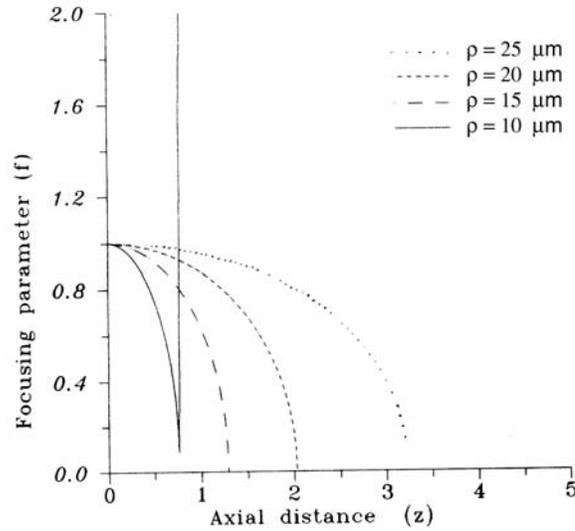
**Figure 3.** Variation of beam width parameter ( $f$ ) with axial distance ( $z$ ) for different values of transverse distance ( $\rho$ ) for parabolic profile fiber corresponding to non-saturating non-linearity. Here  $\epsilon_{CO} = 2.25$ ,  $\epsilon_S = 0.01125$ ,  $\epsilon_{NL} = 9 * 10^{-22}$ ,  $\lambda = 1.55 \mu\text{m}$ ,  $E_0 = 1 * 10^{10}$ ,  $\Delta = 0.001$ ,  $r_0 = 25 \mu\text{m}$  and  $a_0 = 25 \mu\text{m}$ .
