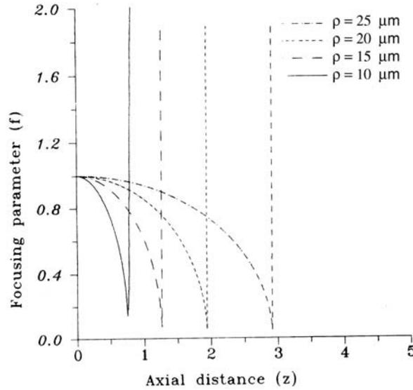
**Figure 2.** Axial dependence of the beam width focusing parameter ( $f$ ) on axial distance ( $z$ ) for different values of initial transverse distance ( $\rho$ ), for step-index fiber in the case of non-saturating non-linearity. Here  $\epsilon_{CO} = 2.25$ ,  $\epsilon_{NL} = 9 * 10^{-22}$ ,  $E_0 = 1 * 10^{10}$ ,  $\epsilon_S = 0.01125$ ,  $\lambda = 1.55 \mu\text{m}$ ,  $\Delta = 0.001$ ,  $r_0 = 25 \mu\text{m}$  and  $a_0 = 25 \mu\text{m}$ .
