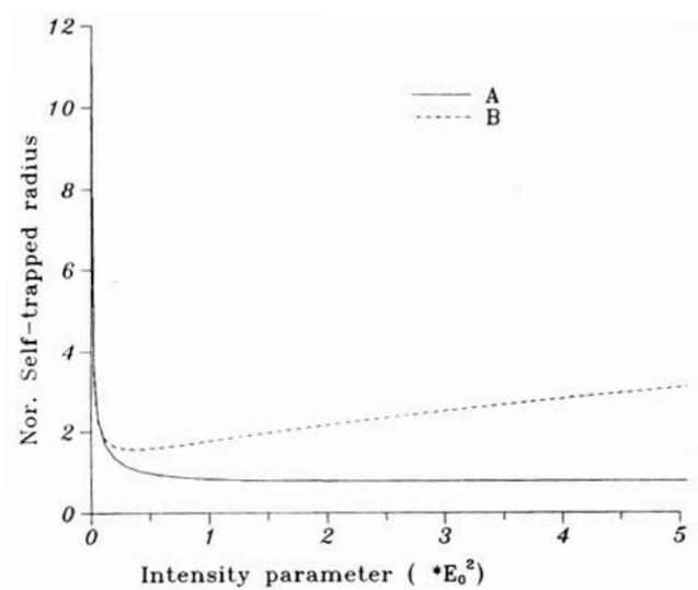
**Figure 7.** Normalised self-trapped radius of beam ( $\omega r_0/C$ ) dependence on beam intensity parameter ( $E_0^2$ ). Curve A for the present non-paraxial analysis and curve B for the paraxial ray approximation. Here  $\epsilon_{CO} = 2.25$ ,  $\epsilon_{NL} = 9 * 10^{-22}$ ,  $\lambda = 1.55 \mu\text{m}$  and  $r_0 = 25 \mu\text{m}$ .
