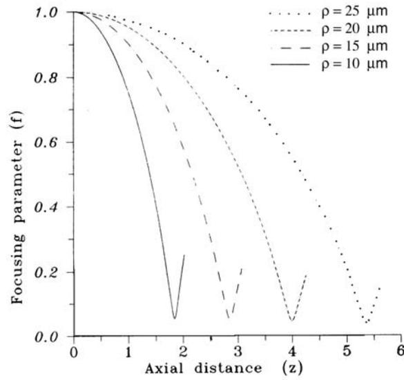
**Figure 5.** Variation of beam width parameter ( $f$ ) with the axial distance ( $z$ ) for the saturating Kerr non-linearity in the case of step-index profile propagation. Here  $\epsilon_{CO} = 2.25$ ,  $\epsilon_S = 0.01125$ ,  $\epsilon_{NL} = 9 \times 10^{-22}$ ,  $E_0 = 1 \times 10^{10}$ ,  $\lambda = 1.55 \mu\text{m}$ ,  $\Delta = 0.001$ ,  $r_0 = 25 \mu\text{m}$  and  $a_0 = 25 \mu\text{m}$ .
