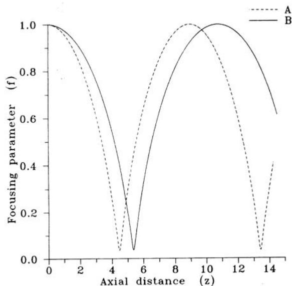
**Figure 4.** Oscillatory behaviour of the focusing parameter ( $f$ ) with the axial distance ( $z$ ) for saturating Kerr non-linearity. Curve A denotes the step-index profile fiber and Curve B the parabolic profile fiber. Here  $\epsilon_{CO} = 2.25$ ,  $\epsilon_S = 0.01125$ ,  $\epsilon_{NL} = 9 * 10^{-22}$ ,  $\lambda = 1.55 \mu\text{m}$ ,  $E_0 = 1 * 10^{10}$  and  $a_0 = 25 \mu\text{m}$ .
