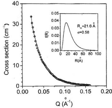
**Figure 2.** Small angle neutron scattering distribution from ferrofluid sample comprised of the nano-particles. Fitted pattern (continuous line) assuming spherical shape and log-normal particle size distribution with mean diameter  $D_m = 43.6 \text{ \AA}$  and standard deviation  $\sigma = 0.58$  is also shown. In the inset is shown the particle size distribution.
