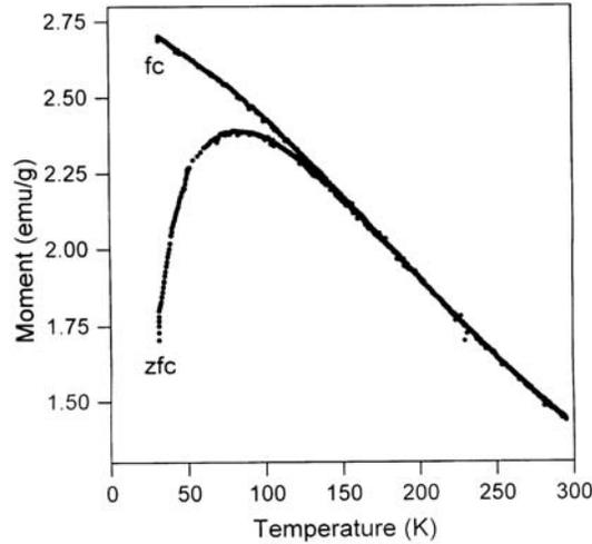
**Figure 5.** Magnetization–temperature curve recorded in zfc and fc modes (cf. text) in an external magnetic field of 50.8 gauss.
