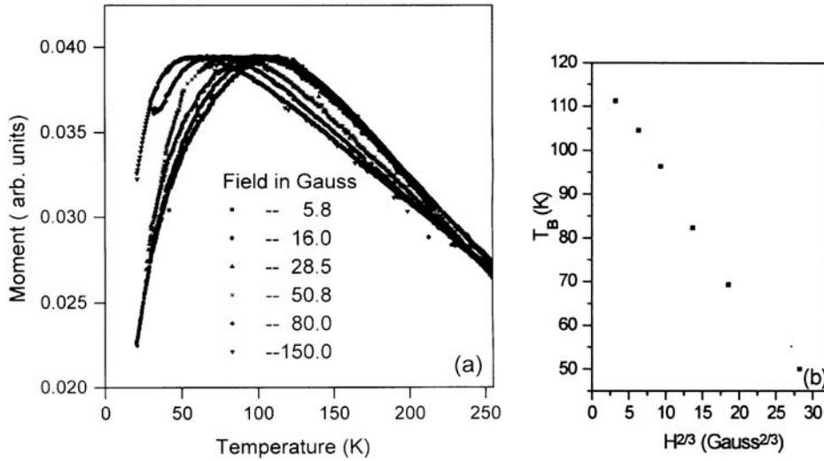
**Figure 6.** (a) Magnetization-temperature curves recorded in zfc mode in the presence of different external magnetic fields  $H$  and (b) a plot of blocking temperature  $T_B$  vs.  $H^{2/3}$ .
