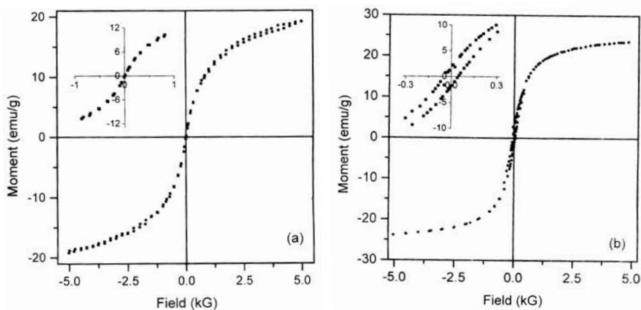
**Figure 3.** Magnetization–field curves recorded at sample temperatures (a) 295 K and (b) 21 K. Insets to figures show expanded low field region.
