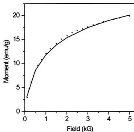
**Figure 4.** Magnetization–field curve recorded at 295 K along with Langevin function fitting.
