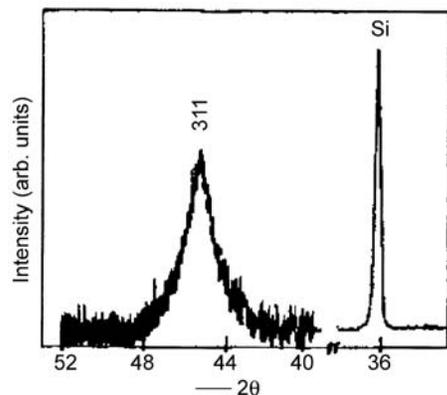
**Figure 1.** The 311 reflection line from the X-ray diffraction pattern of the nano-particle sample recorded with  $\text{FeK}\alpha$  radiation (a reflection line of diffraction pattern of a bulk particle sample of Si is shown for comparison).
