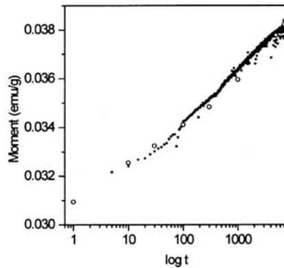
**Figure 7.** Magnetization  $M$  as a function of logarithm of observation time  $t$  recorded in zfc mode at a sample temperature of 21 K. Calculated points taking into consideration the particle size distribution and two values for magnetic anisotropy constant (see text) are also shown for some observation times by open circles.
