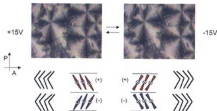
**Figure 12.** Switching behaviour of compound **7** as observed between crossed polarisers. The texture was obtained upon cooling from the isotropic liquid under an applied electric AC field of  $50 \text{ V } \mu\text{m}^{-1}$  (200 Hz). The extinction crosses coincide with the crossed polarisers and do not rotate when an electric field is applied. Below the textures the proposed organisation of the molecules in the different switched states are shown [38].
