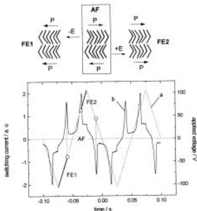
**Figure 4.** Typical switching current response curve on applying a triangular wave voltage as measured for an antiferroelectric B2-type mesophase. a = triangular wave voltage, b = switching current response curve ( $6 \mu\text{m}$  polyimide-coated ITO-coated cell) [13].
