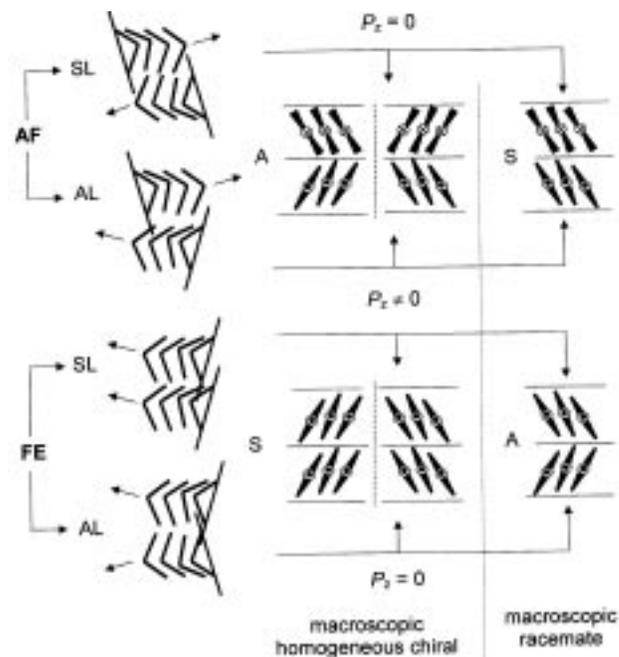
**Figure 16.** Views of the eight possible supermolecular isomers of polar double-tilted  $\text{SmC}_G$  phases [55]. At the left AF and FE organisations are shown. For each isomer a syn-leaning (SL) and antileaning (AL) correlation is possible. All pictures at the right represent orthogonal views upon these arrangements;  $P_z$  = out-of-plane polarisation component [55].
