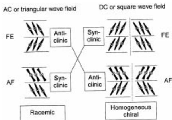
**Figure 13.** Influence of external electric fields on the organisation of FE and AF switching mesophases of bent-core molecules. DC or square wave fields lead to homogeneous chiral structures (synclinic interfaces for FE phases, but anticlinic interfaces for AF phases). AC or triangular wave fields lead to racemic structures (anticlinic interfaces for FE phases, but synclinic interfaces for AF phases).
