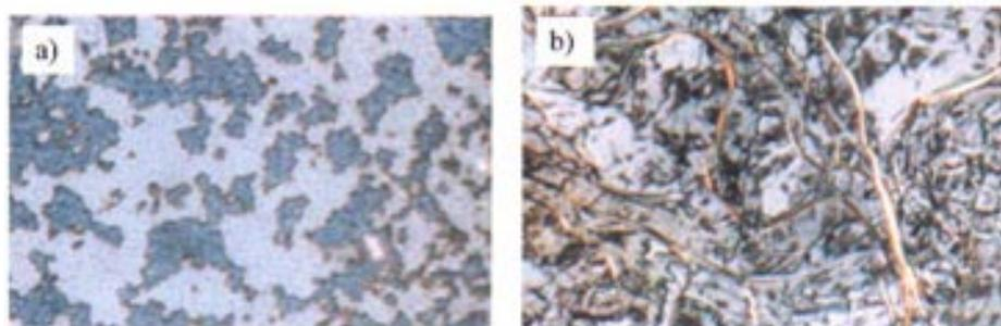
**Figure 19.** Textures of the mesophase of compound **15**. (a) Texture composed of regions with opposite chirality as obtained upon cooling from the isotropic liquid state (the photograph was taken with polariser and analyser slightly uncrossed to distinguish domains of opposite chirality, upon changing the direction of the analyser the brightness of the domains is reversed) and (b) Schlieren texture as obtained upon heating from the crystalline solid state.
