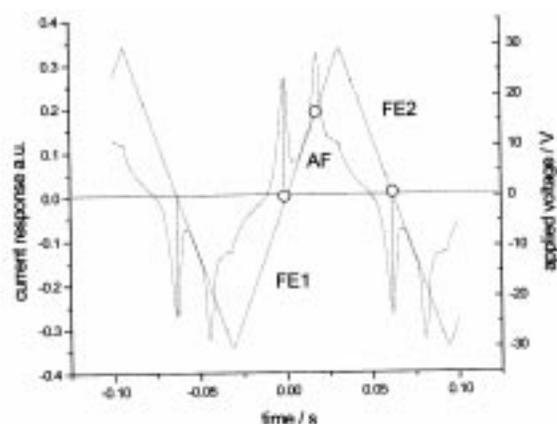
**Figure 17.** Switching current response on applying a triangular wave voltage as recorded for the antiferroelectric switching banana mesophase of compound **13b** ( $6 \mu\text{m}$  polyimide-coated ITO cell) [62].
