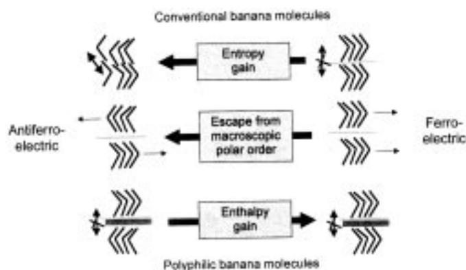
**Figure 14.** The driving forces behind the FE and AF organisation of bent-core molecules. The AF structure is stabilised by the escape from a macroscopic polar order and the entropy gain due to out-of-plane interlayer fluctuations. If the layers are decoupled the importance of the entropy gain is reduced and intermolecular interactions (enthalpy gain) can give rise to a stabilisation of the FE structure.
