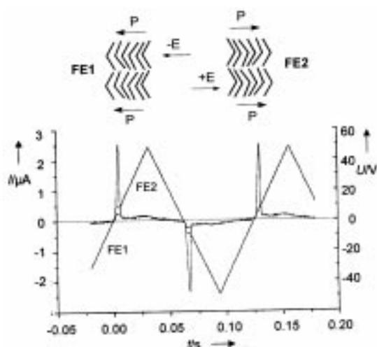
**Figure 10.** Typical switching current response on applying a triangular wave voltage as recorded for the ferroelectric switching banana mesophase of compound **7** ( $10 \mu\text{m}$  non-coated ITO cell) [38].
