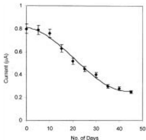
**Figure 11.** Response of P3DT/SA/GOX electrodes as a function of storage time in the presence of glucose (100 mg/dL) in phosphate buffer (pH 7).
