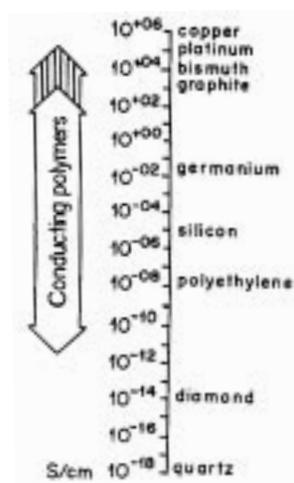
Figure 1. Conductivity chart for various conducting polymers.
