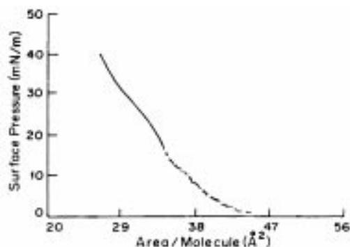
**Figure 6.** Pressure–area isotherm of mixed monolayers of poly-*n*-vinyl carbazole (PNVK) and stearic acid (SA) at a sub-phase temperature of 30°C and pH 7.0.
