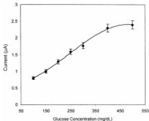
**Figure 10.** Amperometric response of P3DT/SA/GOX LB film in phosphate buffer (pH 7.0) at 0.4 V (bias voltage).
