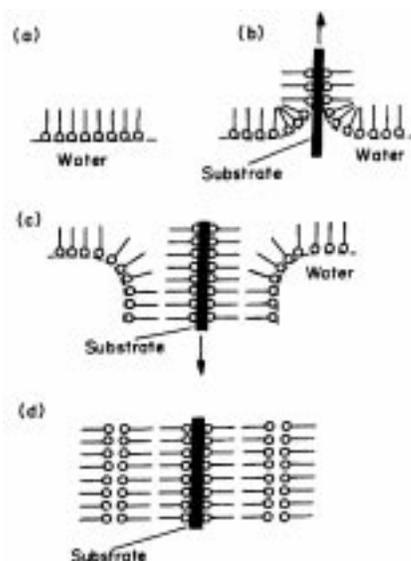
**Figure 4.** Schematic of Y-type deposition in a Langmuir trough. (a) Compressed monolayer of molecules on water surface, (b) deposition of first monolayer withdrawn on hydrophilic substrate, (c) deposition of second monolayer on insertion of hydrophilic substrate, (d) deposition of third monolayer in head-to-head and tail-to-tail configuration.
