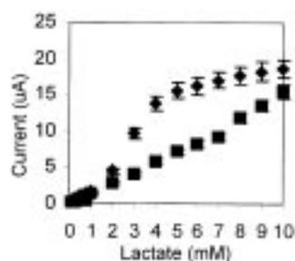
**Figure 5.** Calibration curve for sol-gel/PANI/LDH electrodes as a function of lactate concentration before PVC coating (◆) and after PVC coating (■).
