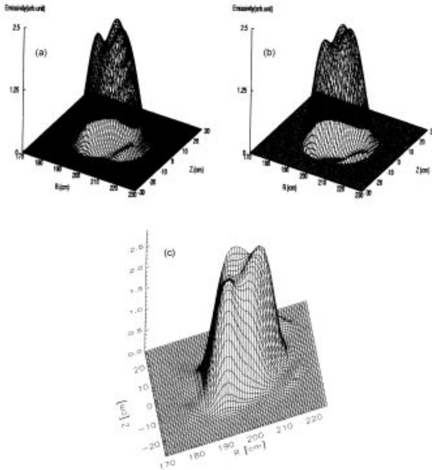
**Figure 7.** (a) The 3D image of the W7-AS Stellarator srx data using Bessel function as the base function for radial expansion, (b) when Zernicke polynomial was used as base function and (c) 3D image supplied by Weller and Klose [15].
