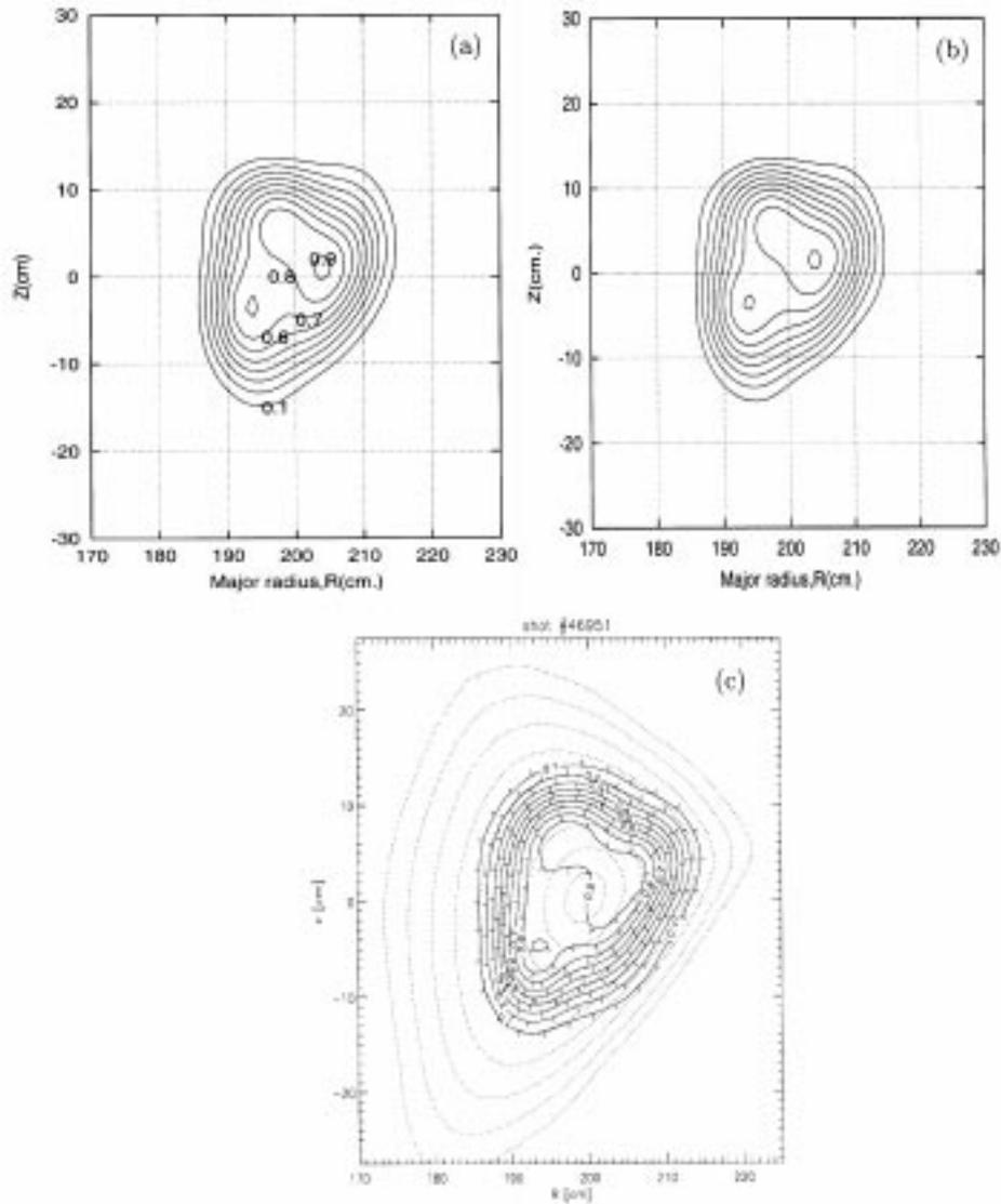
**Figure 6.** Reconstructed image of srx emissivity of W7-AS Stellarator (a) using Bessel function as the base function for radial expansion, (b) using Zernicke polynomial as the base function for radial expansion and (c) is the reconstructed 2D image supplied by Weller and Klose [15].
