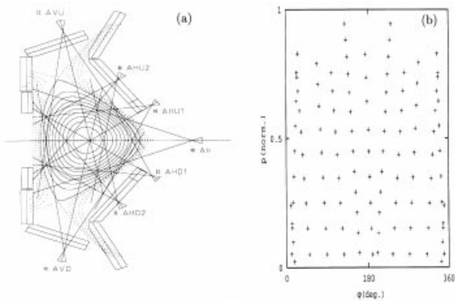
**Figure 3.** (a) The arrangement of 7 fan arrays to be installed in SST-1. (b) Plot of  $(p, \phi)$ -coordinates of 115 chords in 7 arrays.
