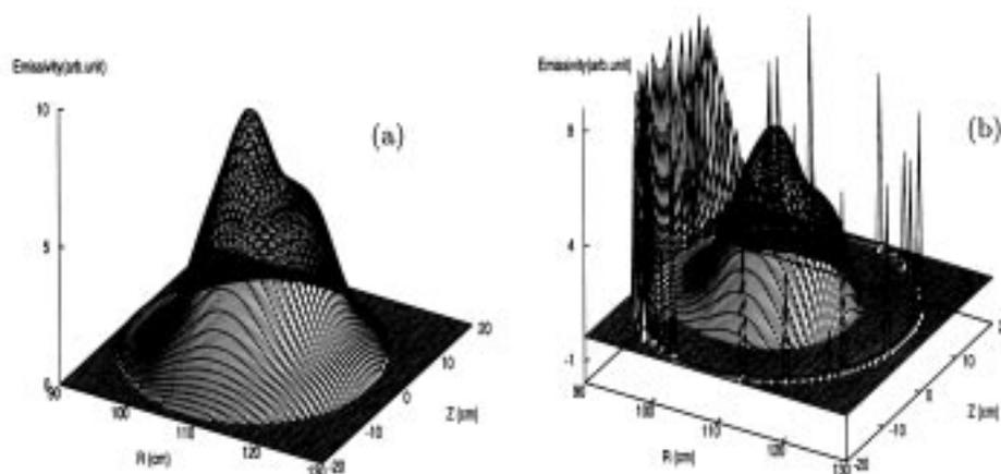
**Figure 5.** (a) The 3D image of Kadomtsev's model for saw-tooth oscillation reconstructed with the code using Zernicke polynomial as the base function for radial expansion when 180 virtual chords were used. (b) The 3D image reconstructed with that code when no virtual chord was used. The spikes and small negative emissivity is obvious at the edge region.
