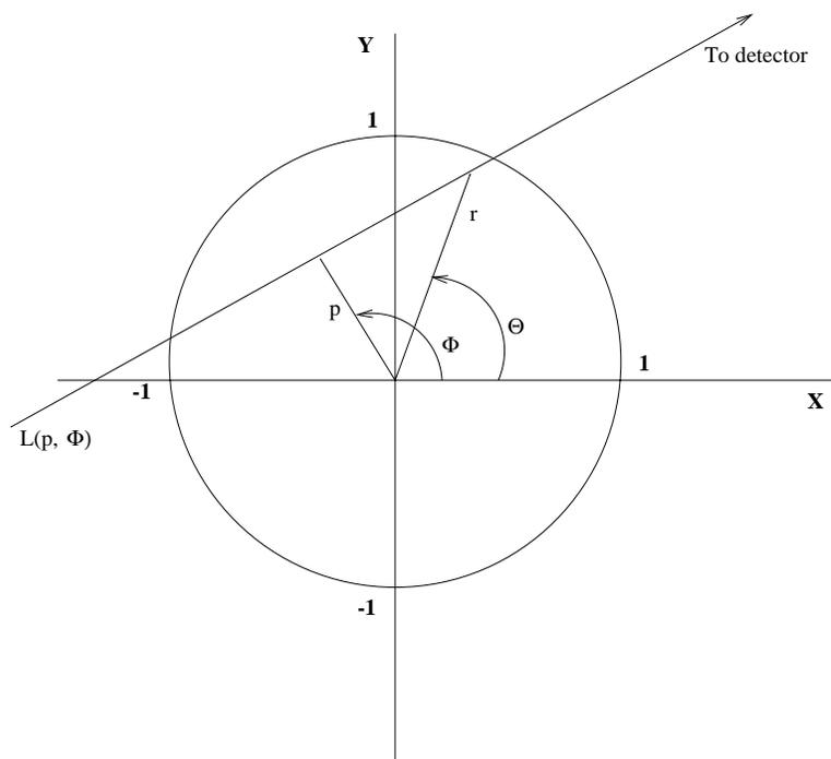
**Figure 1.** Detectors integrate the local emissivity,  $g(r, \theta)$  along lines-of-sight,  $L$  defined by  $(p, \phi)$ . The emitting region must be completely contained within the circular region.
