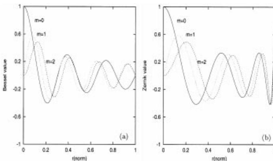
**Figure 2.** (a) The Bessel function with  $l = 6$  and  $m = 0, 1, 2$ . (b) The Zernike polynomial for the same  $l$  and  $m$  values. Note the boundary values of the two functions. For details, see text.
