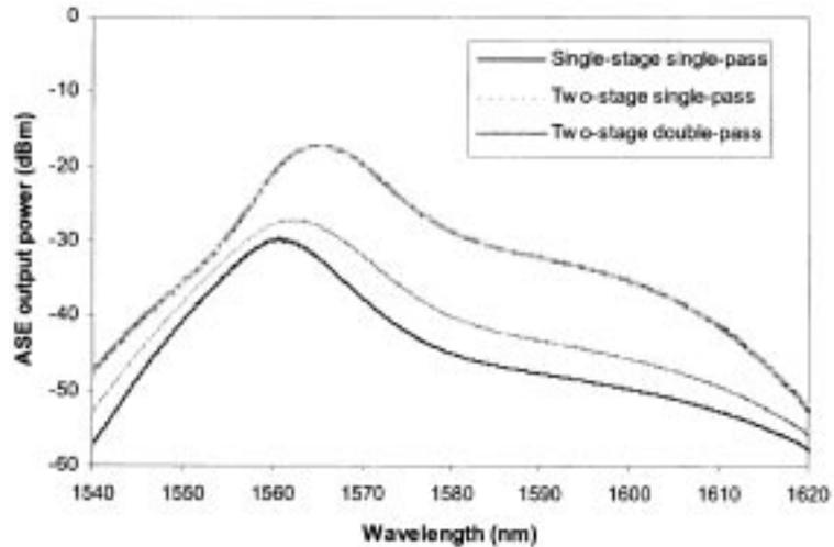
Figure 2. ASE spectra of the L-band EDFA while the total pump power is fixed at 92 mW. For the dual-stage amplifiers, pump 1 and pump 2 are fixed at 35 mW and 57 mW, respectively.
