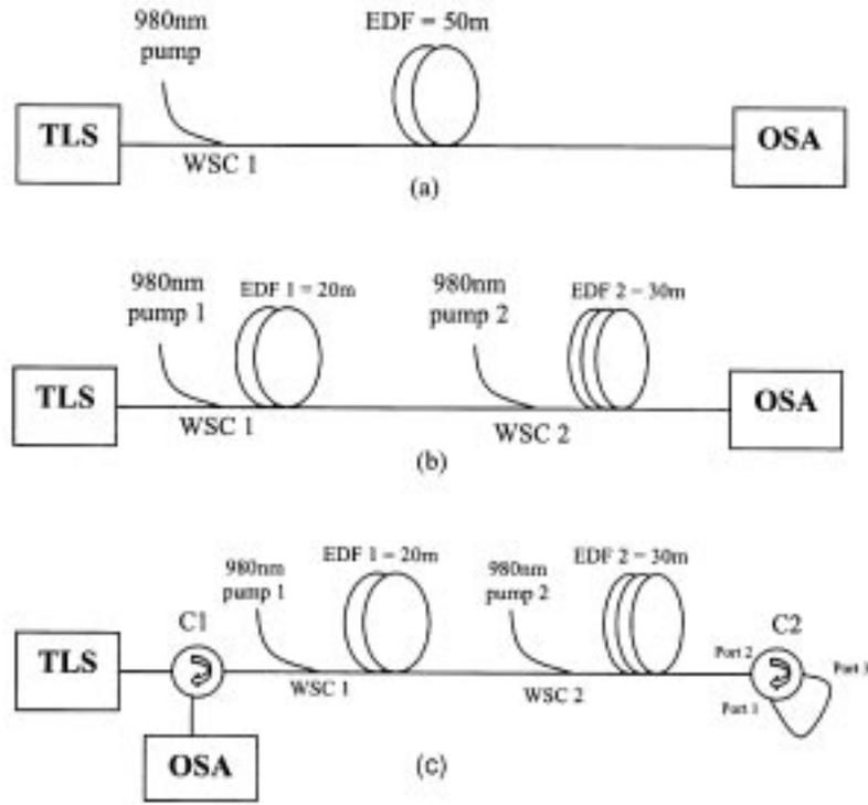
Figure 1. Configuration of the L-band EDFAs in (a) single-stage single-pass, (b) two-stage single-pass and (c) two-stage double-pass.
