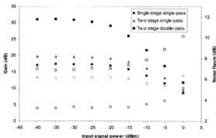
**Figure 3.** Gain (filled) and noise figure (open) as a function of input signal power.
