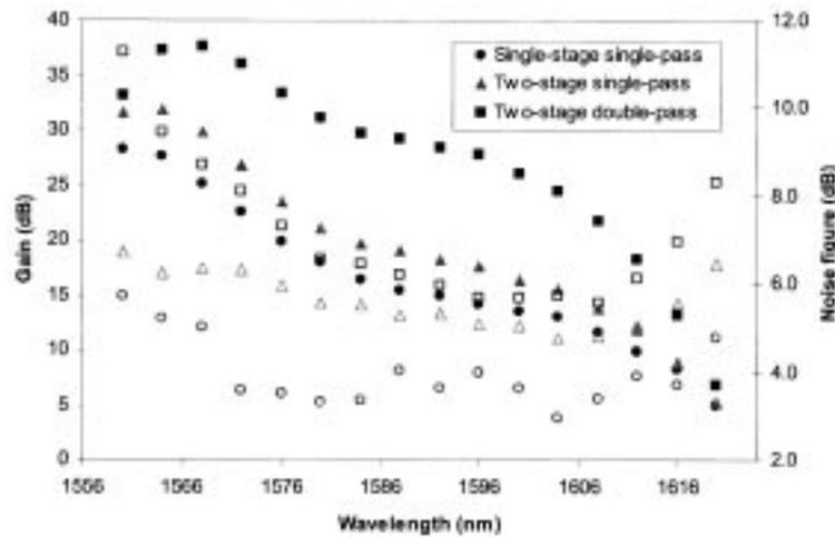
Figure 4. Gain (filled) and noise figure (open) as a function of input signal wavelength.
