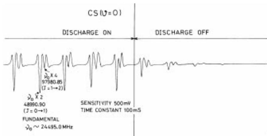
**Figure 2.**  $J = 0 \rightarrow 1$  and  $J = 1 \rightarrow 2$  transitions of  $^{12}\text{C}^{32}\text{S}$  at 48990.90 MHz and 97980.85 MHz respectively using the second and fourth harmonic of klystron fundamental frequency (lock-in amplifier sensitivity = 500 mV, time constant = 100 mS).
