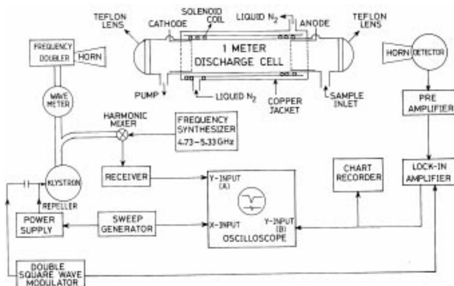
Figure 1. Block diagram of the millimeterwave spectrometer.
