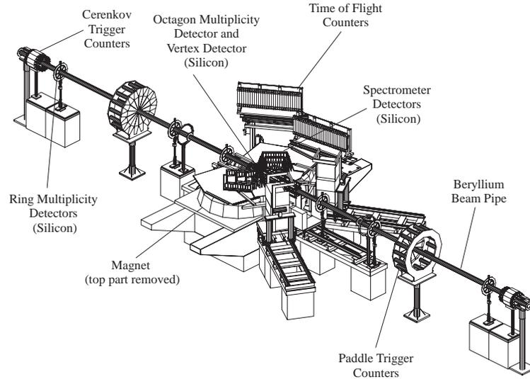
**Figure 1.** Schematic drawing of the PHOBOS setup. See text for details.
