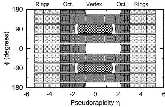
**Figure 2.** The geometrical acceptances of the ring (light), octagon (medium) and inner vertex (checker board) detectors for particles emitted from the nominal interaction point are shown as a function of  $\eta$  and azimuthal angle  $\phi$ .
