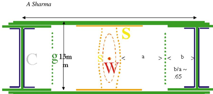
**Figure 8.** Schematic of the drift tubes of CMS. Continuous lines represent electrodes, dotted lines represent equipotential surfaces.
