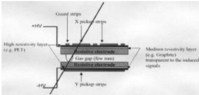
**Figure 14.** Schematic of a resistive plate chamber.
