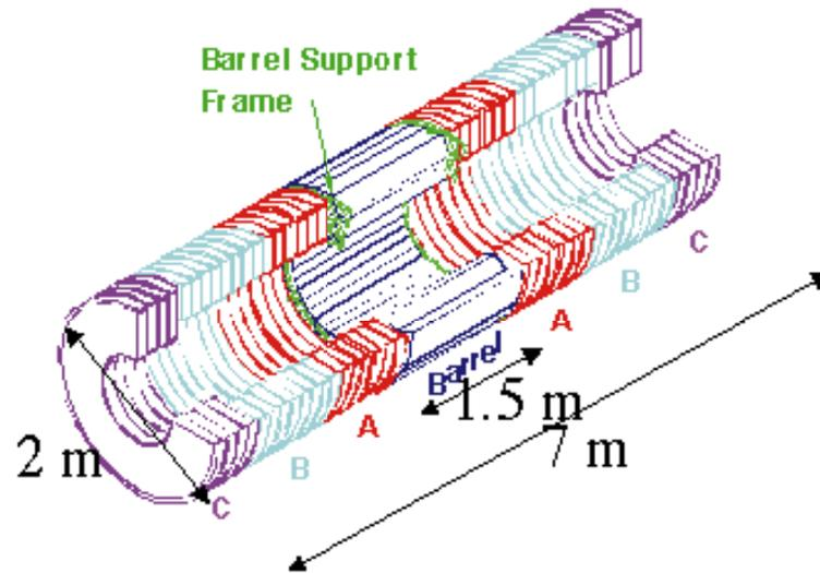
Figure 7. Schematic of the ATLAS TRT detector.
