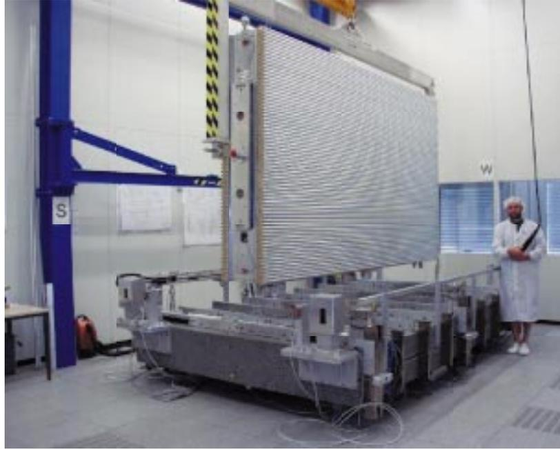
Figure 6. A finished MDT module at MPI, Germany.
