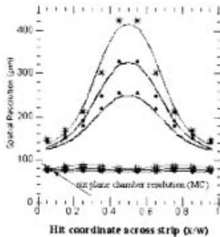
Figure 12. Resolution along readout strips for CSCs.
