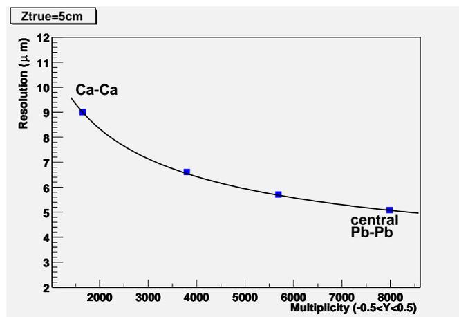
**Figure 5.** Resolution on the primary vertex  $Z$  coordinate as a function of the multiplicity in the central unit of rapidity. The full line is a fit with the function  $\sigma_z = B + A/\sqrt{dN_{ch}/d\eta}$  with  $A = 292$  and  $B = 1.8$ .
