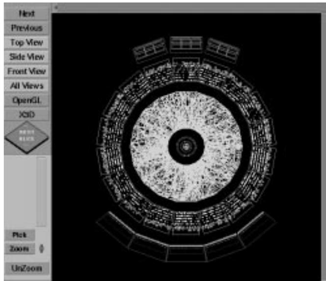
**Figure 4.** AliRoot event display. Particles are generated with a polar angle  $\theta$  in the range  $85 < \theta < 95$  with a density corresponding to the maximum foreseen value. Starting from the beam axis, ITS, TPC, TRD and TOF are displayed. PHOS and HMPID are below and above the beam axis respectively.
