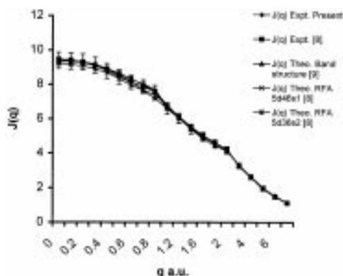
**Figure 2.** Comparison of the present results of Ta with experimental results [8] and with theoretical values based on RFA model [8] and band structure [9] calculations.
