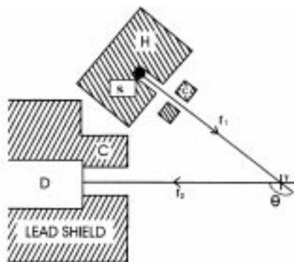
**Figure 1.** Schematic layout of the geometry and shielding arrangement. T - target; S - source; C - collimator; D - HPGGe detector; H - Source collimator;  $r_1$  - source to target distance;  $r_2$  - target to detector distance.
