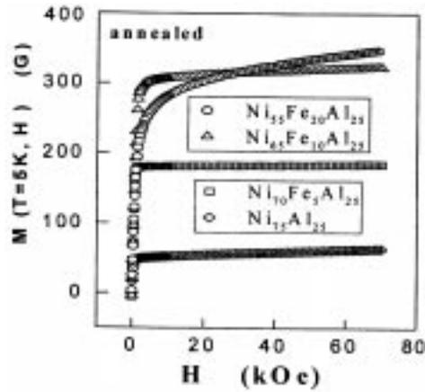
Figure 2. Magnetisation  $M$  at 5 K as a function of field  $H$ .
